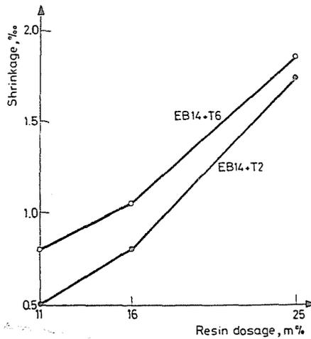
Fig. 7. Final shrinkage vs. resin dosage
