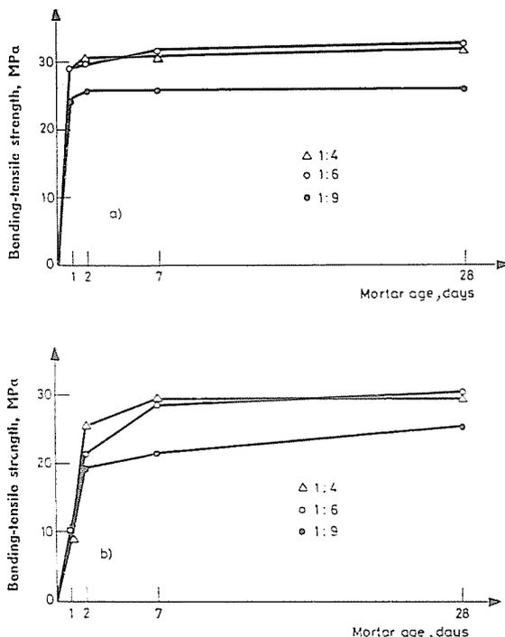
Fig. 2. Bending-tensile strength of epoxy resin vs. time at ambient temperature a) with T2; b) with T6
