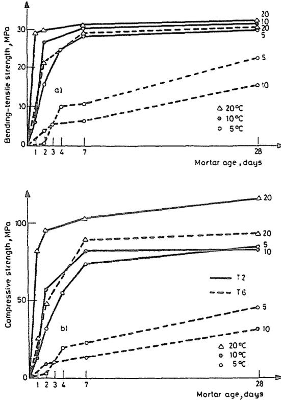
Fig. 4. Effect of temperature on the hardening process of epoxy mortar at 1 : 6 resin to sand ratio; a) bending-tensile strength; b) compressive strength
