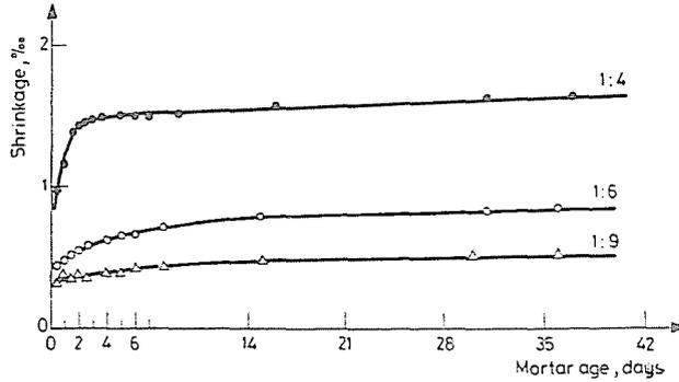
Fig. 6. Shrinkage vs. time for amine-type cross-linking agent T2
