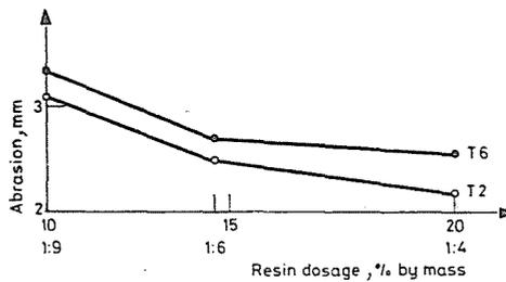
Fig. 8. Abrasion rate vs. resin dosage
