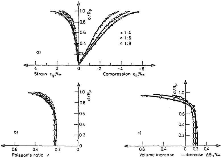
Fig. 11. Deformation, volume change and Poisson's ratio of 39-day prisms made with T2 vs.  $\sigma/R_p$
