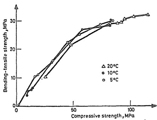
Fig. 5. Bending-tensile vs. compressive strength. Resin: sand = 1 : 6. Stored at 5 °C, 10 °C and 20 °C, resp.
