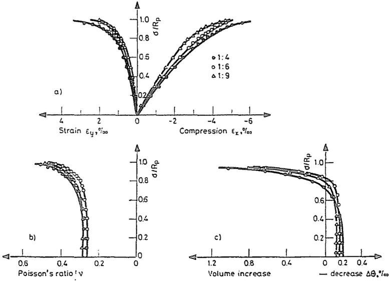
Fig. 10. Deformation, volume change and Poisson's ratio of 7-day prisms made with T2 vs.  $\sigma/R_p$
