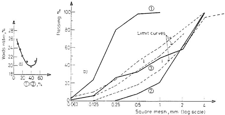
Fig. 1. Aggregate. a) Variation of the voids ratio with the proportion of both fractions; b) grading curve (3) experimentally determined from limit curves, initial aggregate fractions (1) and (2) and from the voids minimum
