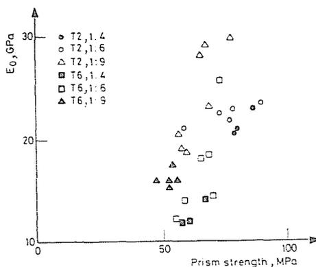
Fig. 14. Initial modulus of elasticity in compression vs. prism strength
