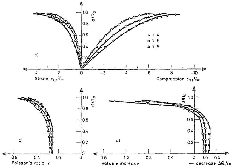
Fig. 12. Deformation, volume change and Poisson's ratio of 28-day prisms made with T6 vs.  $\sigma/R_p$
