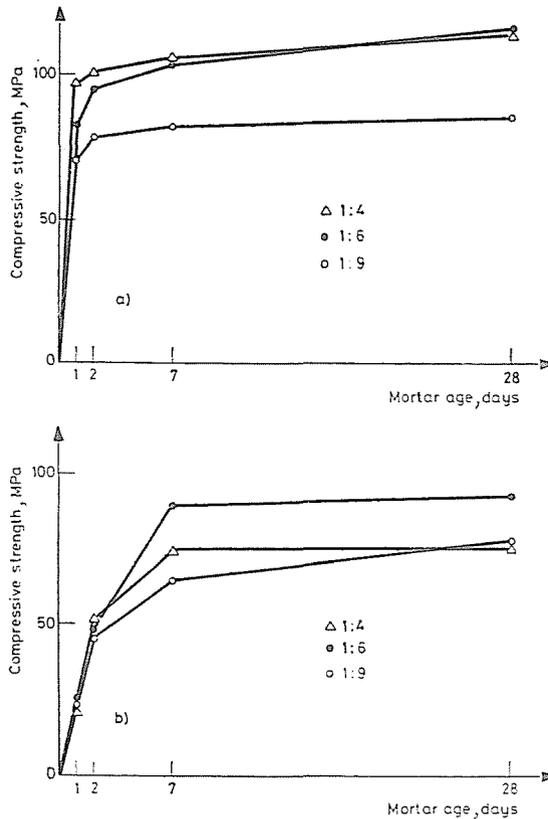
Fig. 3. Compressive strength of epoxy resin vs. time at ambient temperature a) with T2; b) with T6
