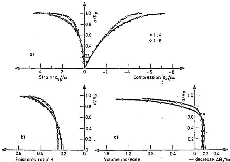
Fig. 9. Deformation, volume change and Poisson's ratio of 1-day prisms made with T2 vs.  $\sigma/R_p$
