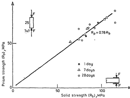
Fig. 13. Prism strength vs. solid strength
