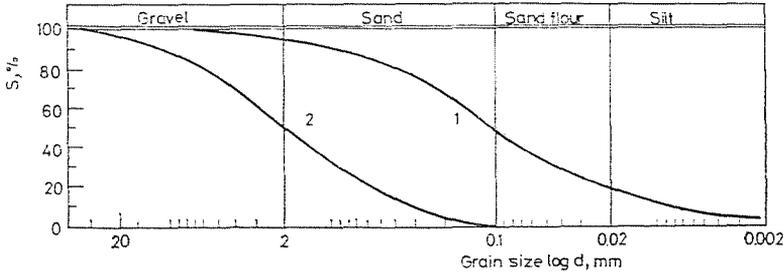
Fig. 5. 1. Grain size distribution of the soil sample taken from the site. 2. Grain size distribution of the catchwater drain material
