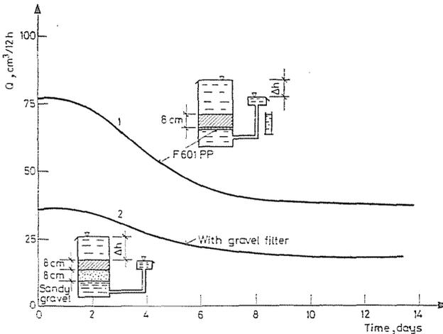
Fig. 6. Model test on soil taken from the site: 1. with fabric F 601; 2. with the drain material
