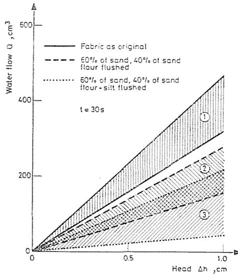
Fig. 4. Permeability change of fabrics due to the trapped soil grains
