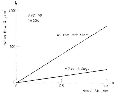
Fig. 7. Permeability change due to grains trapped in the fabric
