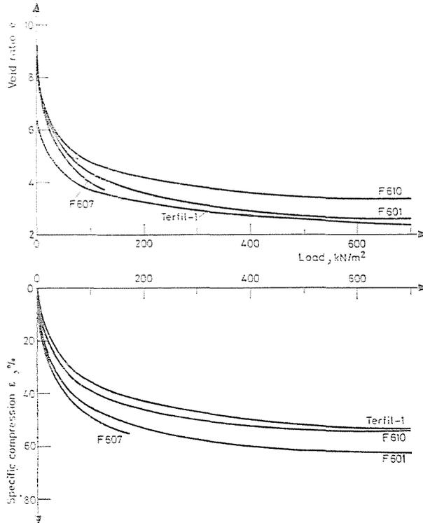
Fig. 2. Compression curves of fabrics
