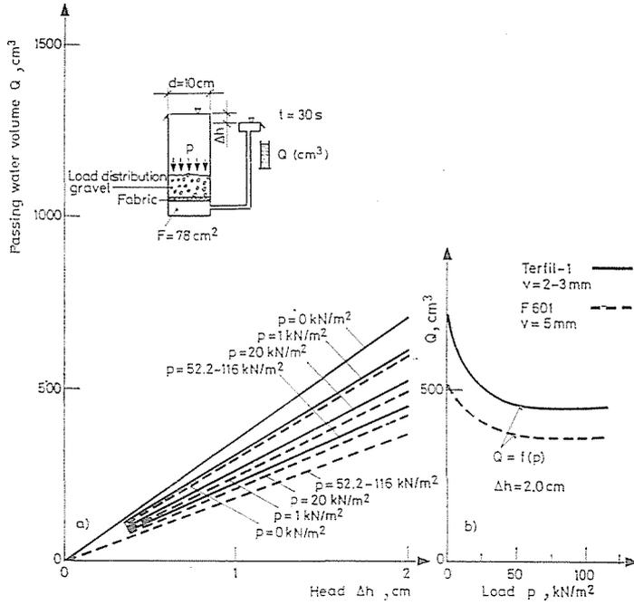
Fig. 3. Permeability change of fabrics vs. load
