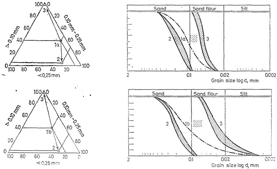
Fig. 1. Vibration-water flushing test results on fabrics. 1/a. 1/b. Grain size distribution curves of the original soil. 2. Range of grain size distribution of the fabric residue. 3. Range of grain size distribution curves of the passing material
