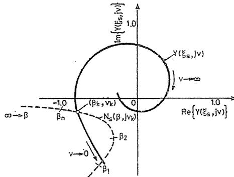
Fig. 3. Nyquist curve and curve of the describing function
