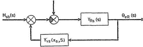
Fig. 2. Flowchart of water level control
