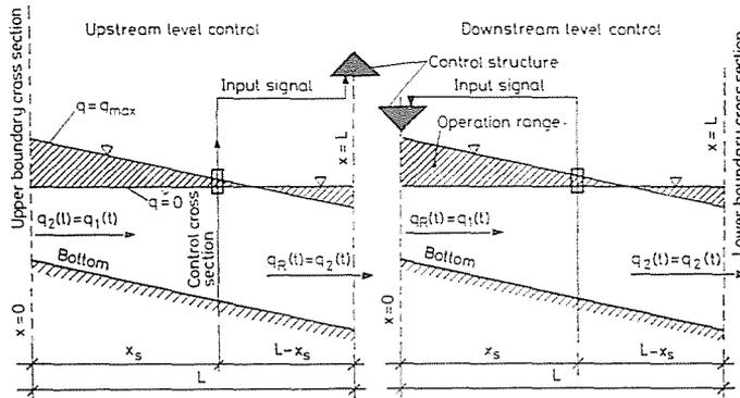
Fig. 1. Schemes of water level control systems
