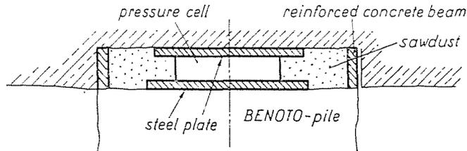
Fig. 9. Placing pressure cells between the beam and the pile head
