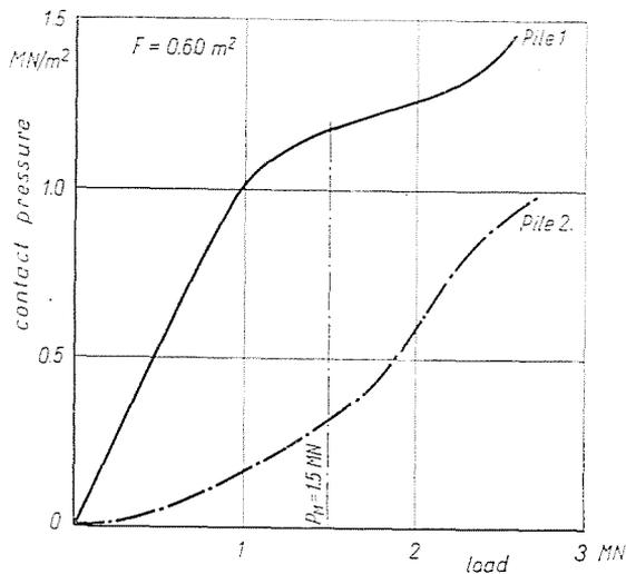
Fig. 3. Base pressure versus load
