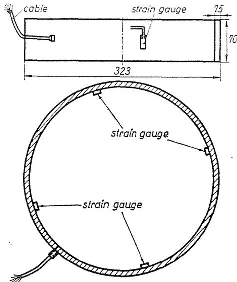
Fig. 8. Sketch of a pressure cell
