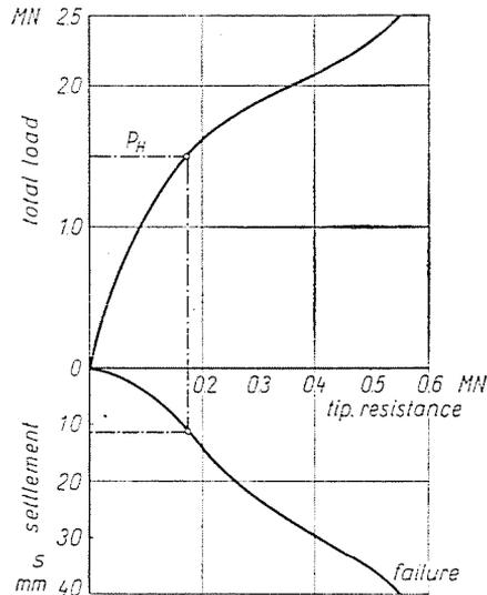
Fig. 7. Relationship between tip resistance, settlement and pile load (pile No. 2)
