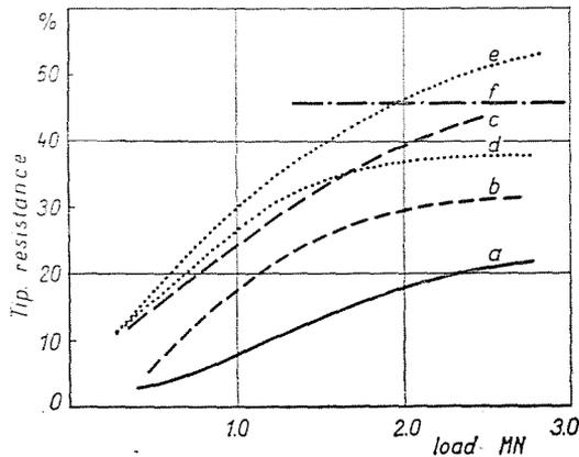
Fig. 5. Percentage distribution of the pile load.  $P_t$  — total pile reaction,  $P_c$  — tip resistance,  $P_k$  — skin friction, a — pile No. 2, b — Kaufman's measurement, pile  $l = 19.8$  m, c — Kaufman's measurement, pile  $l = 20.1$  m, d — slurry trench wall, Óbuda, e — slurry trench wall, Újpalota,  $l = 6.8$  m  $F = 2.2 \times 0.55$  m<sup>2</sup>, f — Kaposvár, value calculated for pile No. 2 (according to Meyerhof's formula)
