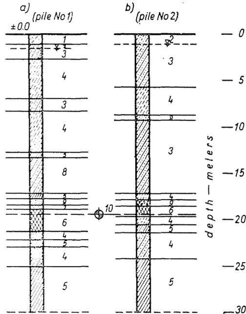
Fig. 1. Boring logs at the site of test piles: a — boring No. 1; b — boring No. 2; 1 — fill; 2 — groundwater table; 3 — silty fine sand; 4 — silt; 5 — clay; 6 — hard clay; 7 — organic; 8 — silty fine sand; 9 — sand, gravel, 10 — plane of the pile base
