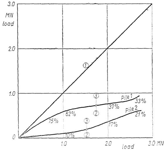
Fig. 4. Distribution of the pile load. 1 — total pile reaction; 2 — tip resistance; 3 — skin friction
