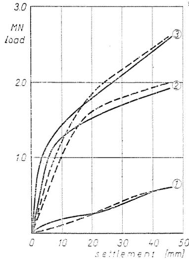
Fig. 6. Variation of skin friction and tip resistance vs. settlement. 1 — tip resistance; 2 — skin friction; 3 — total pile reaction; ---- calculated; ——— measured
