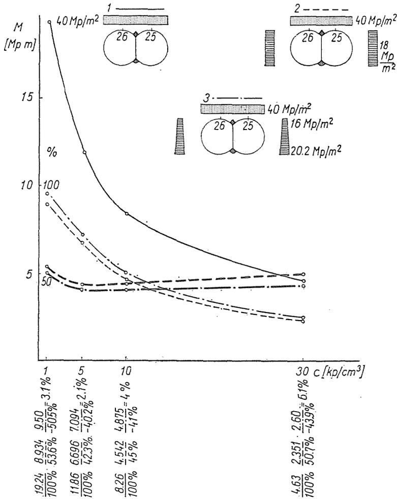
Fig. 6. Maximum positive moment of twin tunnels vs. coefficient of subgrade reaction and distribution of active loads. - - - -  $\Delta M_{1-2}$  = moments in loading case 2 as percentages of case 1; - · - · -  $\Delta M_{1-3}$  = moments in loading case 3 as percentages of case 1
