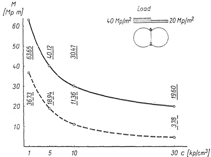
Fig. 14. Bending moments due to asymmetric active load in the column base fixed in the sill beam of the twin tunnel: - - - considering soil bedding of cap and sill beam; ——— omitting soil bedding of cap and sill beam. Remark: Indicated stresses refer to one meter running of tunnel. Their four-fold develops in columns spaced at four meters
