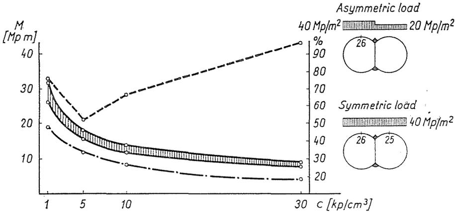
Fig. 8. Positive roof moments vs. load, structural design and coefficient of subgrade reaction
