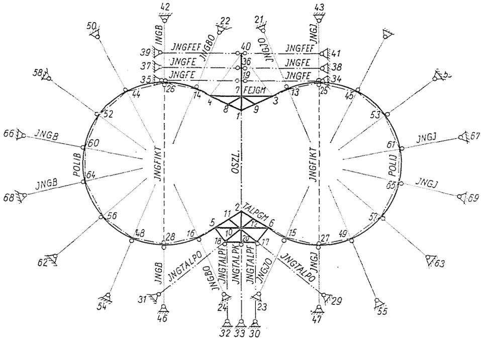
Fig. 2. Structural model of the twin-tunnel cross section of the Budapest-type underground railway station. Remarks: 1. Bars 25—27 and 26—28 INGFIKT with zero bending and compressive rigidities have been applied to ease computer running; 2. Bars crossing in the model are intersecting only if their nodes are numbered
