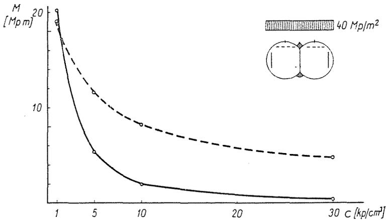
Fig. 3. Roof and springing moments in twin tunnels vs. coefficient of subgrade reaction. ---- roof moment; — moment in the horizontal section
