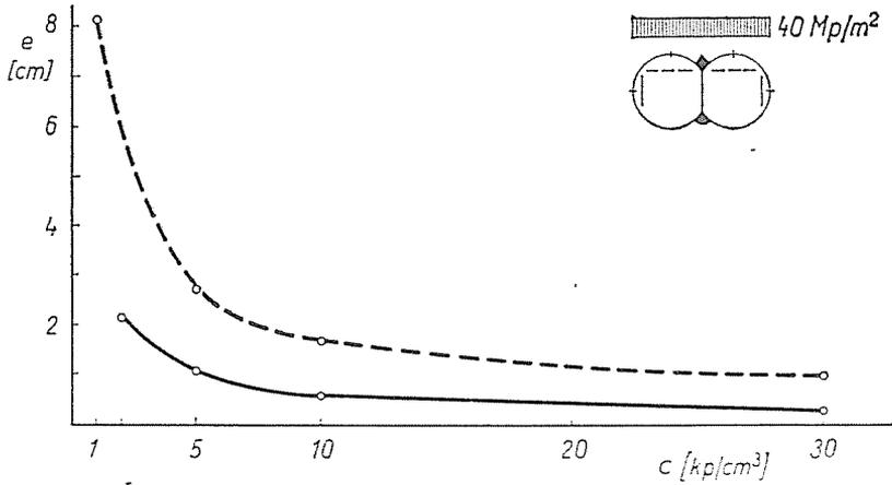
Fig. 4. Vertical and horizontal displacements of the roof and horizontal axis points of a twin tunnel vs. coefficient of subgrade reaction; ----- vertical displacement of roof point, ——— horizontal displacement of horizontal axis point
