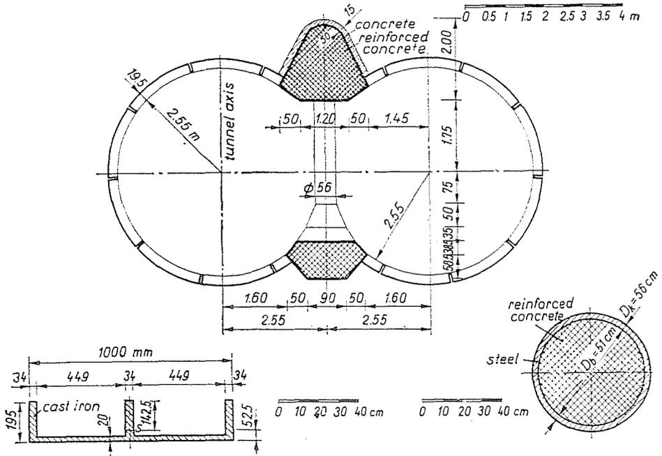
Fig. 1. Twin-tunnel cross section. Cross sections of tubings K-2-L, Sz-2-L N-2-L. Column cross section.  $F = 374 \text{ cm}^2$ ,  $K_{\max} = 2456 \text{ cm}^3$ ,  $K_{\min} = 905 \text{ cm}^3$ ,  $I = 12\,875 \text{ cm}^4$
