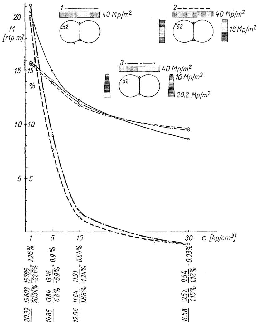
Fig. 7. Maximum negative moment of twin tunnels vs. coefficient of subgrade reaction and distribution of active load. - - - -  $\Delta M$  1-3 = moments in loading case 2 as percentages of case 1; - · - ·  $\Delta M$  1-3 = moments in loading case 3 as percentages of case 1
