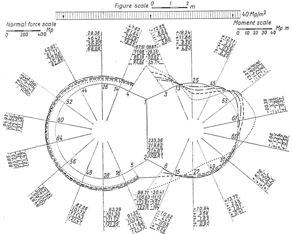
Fig. 5. Normal force and bending moment diagrams for the cross section of a twin tunnel subject to  $40 \text{ Mp/m}^2$  uniform vertical active load for four different bedding coefficients. ....  $c = 1 \text{ kp/cm}^3$ ; -----  $c = 5 \text{ kp/cm}^3$ ; - · - · -  $c = 10 \text{ kp/cm}^3$ ; ———  $c = 30 \text{ kp/cm}^3$
