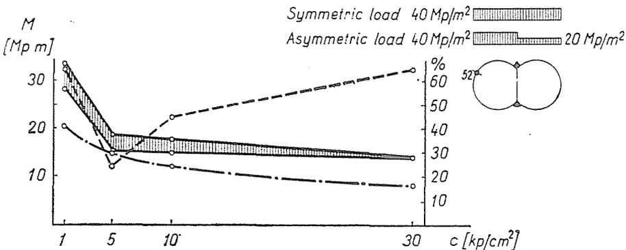
Fig. 9. Negative moments at point 52 vs. load, structural design and coefficient of subgrade reaction
