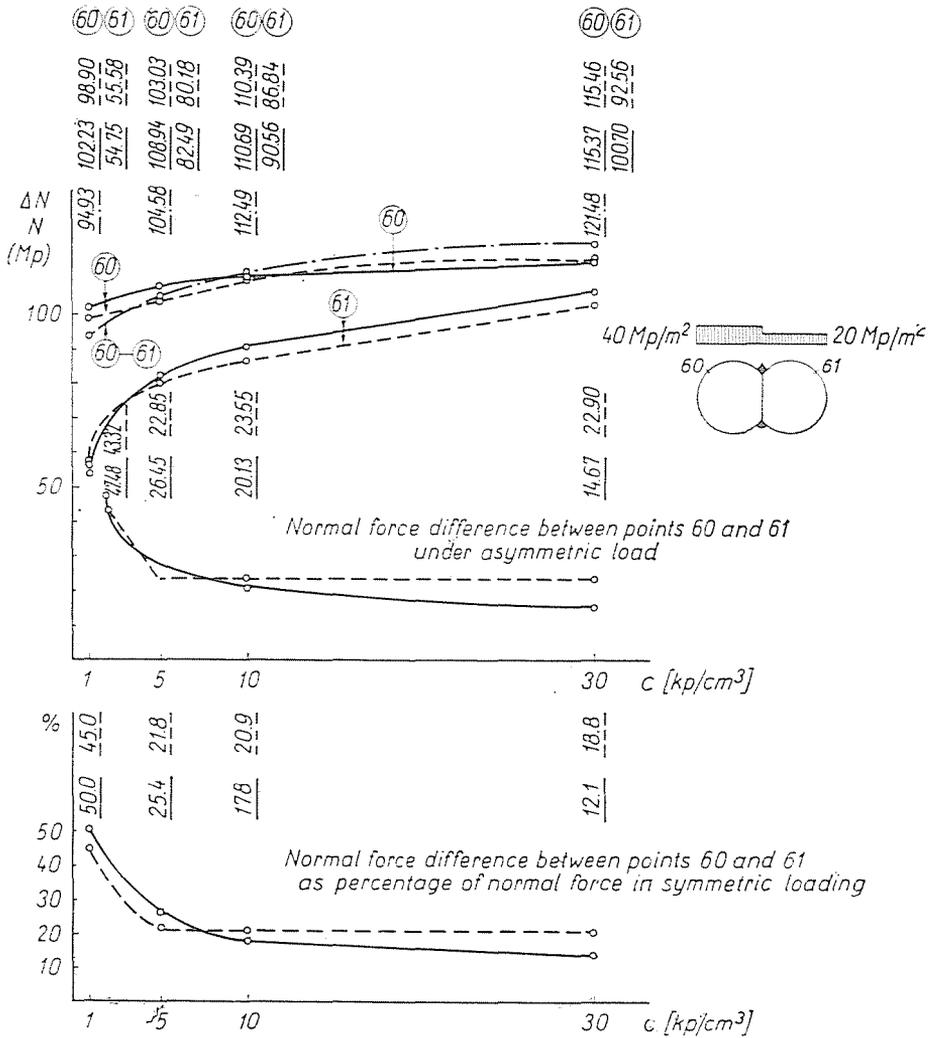
Fig. 12. Normal forces in hinged columns due to asymmetric load vs. coefficient of subgrade reaction at points 60 and 61 symmetric about the twin tunnel column axis: ---- normal force and difference of normal forces for soil-embedded sill and cap beam (asymmetric load); — normal force and difference of normal forces omitting soil bedding of cap and sill beam (asymmetric load); - - - - normal force due to symmetric load at points 60 and 61
