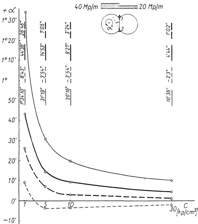
Fig. 13. Deflection from the vertical of the column axis between points 1 and 2 as a function of coefficient of subgrade reaction and structural design: ---- soil-embedded hinged column; — hinged column omitting soil bedding; - - - - clamped column with soil bedding; — clamped column omitting soil bedding. Remark: 1.  $\alpha$  values have been computed from displacements of points 1 and 2; 2. soil bedding refers to cap and sill beam
