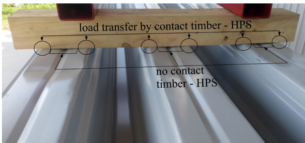
Fig. 9 Load transfer from timber beams on HPS
