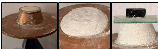
Fig. 2 Schematic representation of flow table test and buildability test
