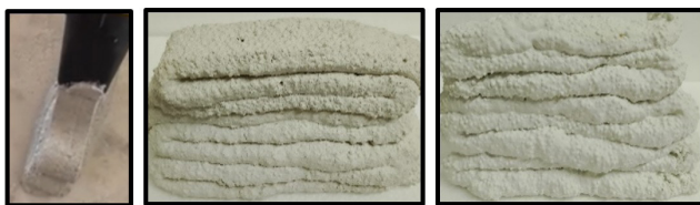
Fig. 1 Extrusion of printable concrete containing EPS
