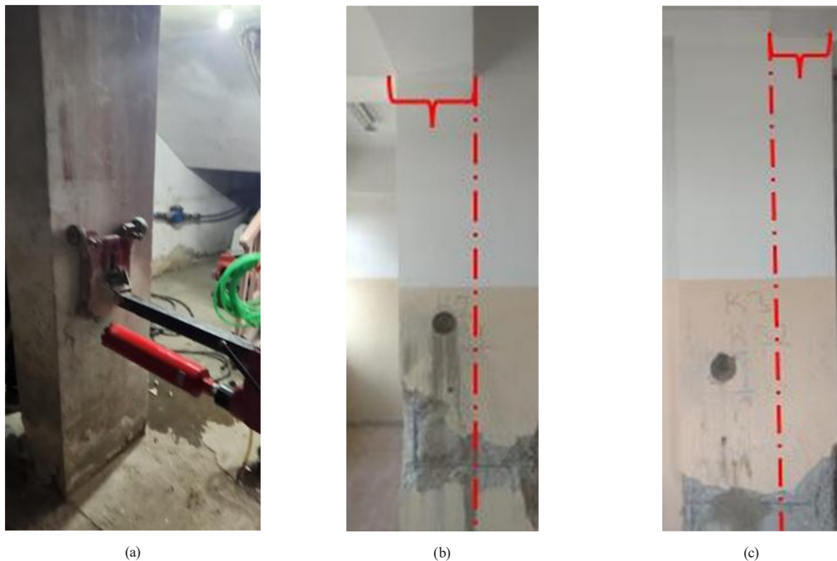
Fig. 1 Core drilling: (a) application; (b) inside; (c) outside the eccentric loading zone
