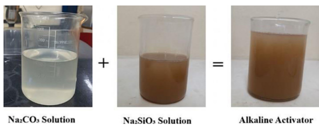
Fig. 2 Alkaline activator preparation
