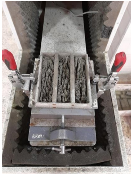
Fig. 2 Steel mold positioned on the shock table
