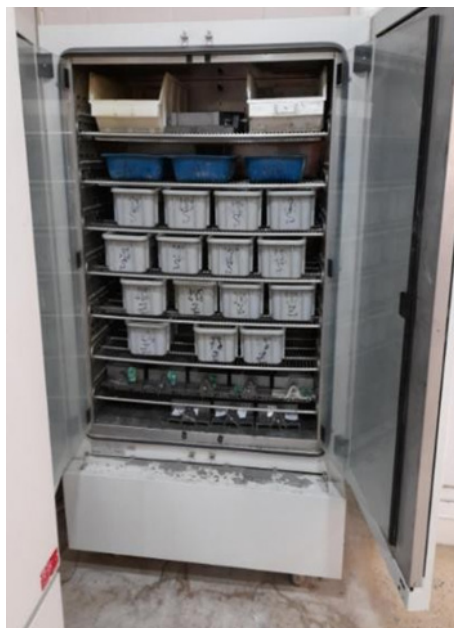
Fig. 3 Specimens in humid chamber (20 °C, 90.5% RH)
