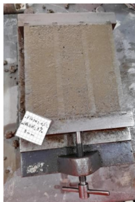
Fig. 1 Steel prismatic mold ( 40 \times 40 \times 160 mm 3 )
