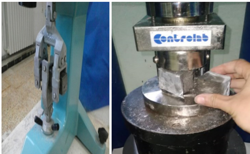
Fig. 6 Tensile tests by bending and compression tests on hardened specimens
