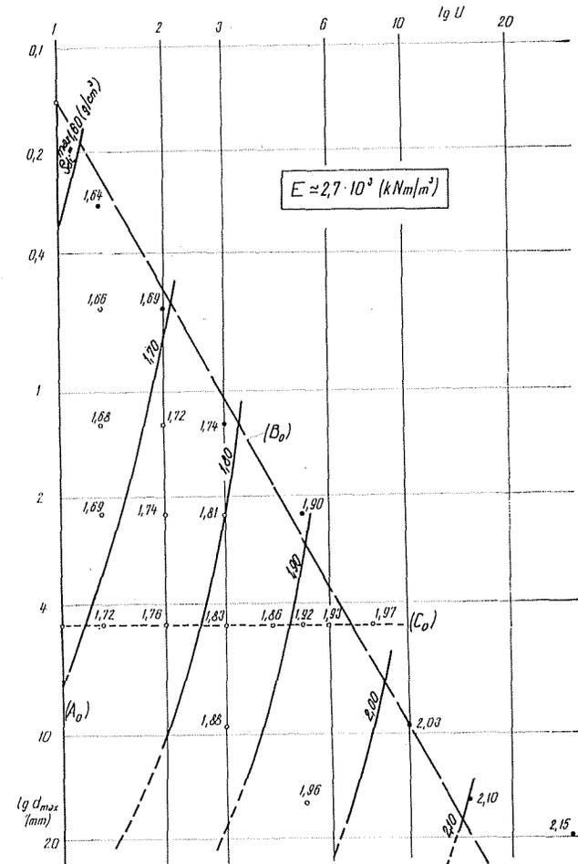
Fig. 8. Bulk densities for  $E = 2.7 \cdot 10^3$  kNm/m<sup>3</sup> compacting work vs. grading
