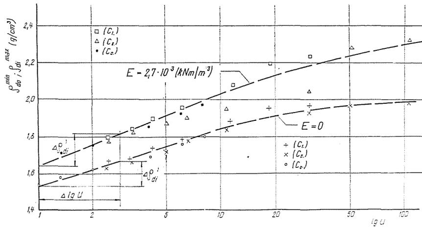
Fig. 13. Density vs. uniformity coefficient for constant compacting works
