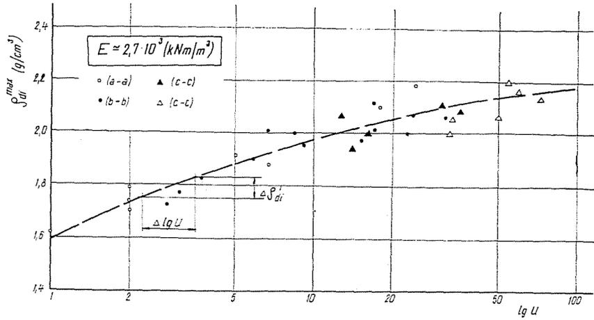
Fig. 16. Density vs. uniformity coefficient for a constant compacting work
