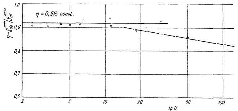
Fig. 14. Relationship between grading and compaction ratio
