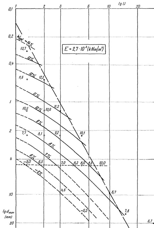
Fig. 9. Optimum water content vs. grading
