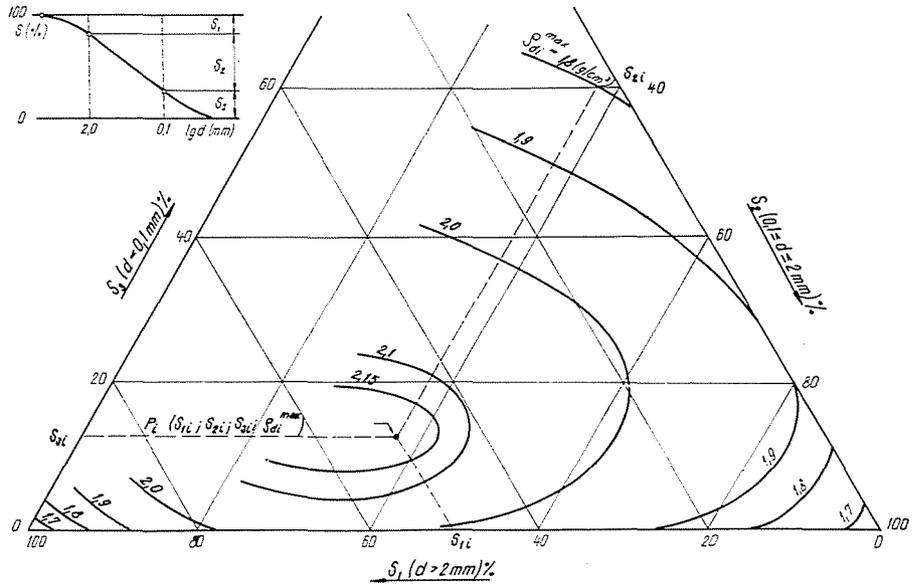
Fig. 18. Density distribution in natural soils due to compacting work, represented in a triangle diagram
