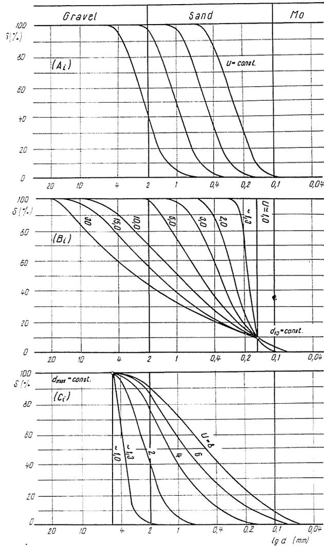
Fig. 2. Three typical groups of tested mixes
