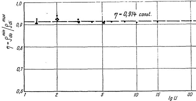
Fig. 12. Relationship between grading and compaction ratio
