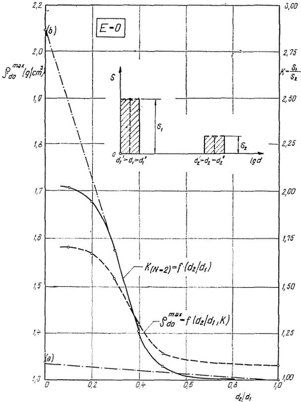
Fig. 19. Relationship between concentration, density and grain size
