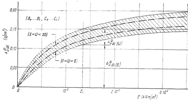
Fig. 11. Density increment vs. grading and compacting work
