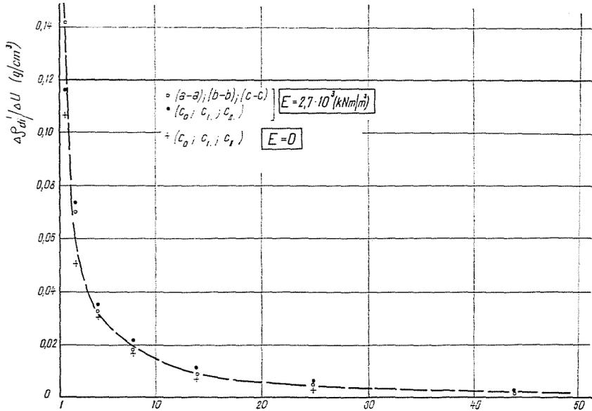
Fig. 17. Derivatives of functions  $\rho_{do}^{max} = f(U)$  and  $\rho_{do}^{min} = f(U)$  vs. uniformity coefficient
