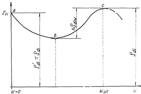
Fig. 7. Shape of the Proctor curve
