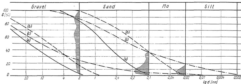
Fig. 15. Grading domains of natural soils and frequency distribution of fractions
