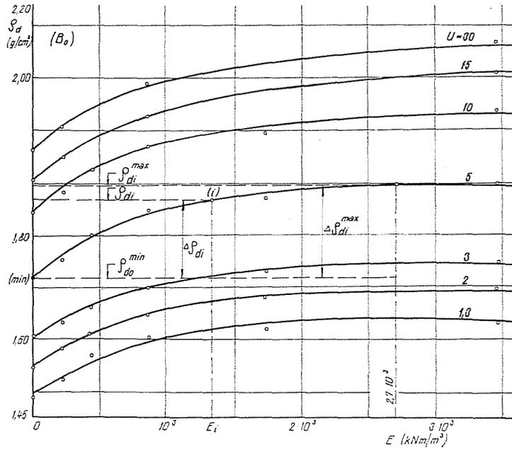
Fig. 10. Density of mix  $B_0$  vs. uniformity coefficient and compacting work
