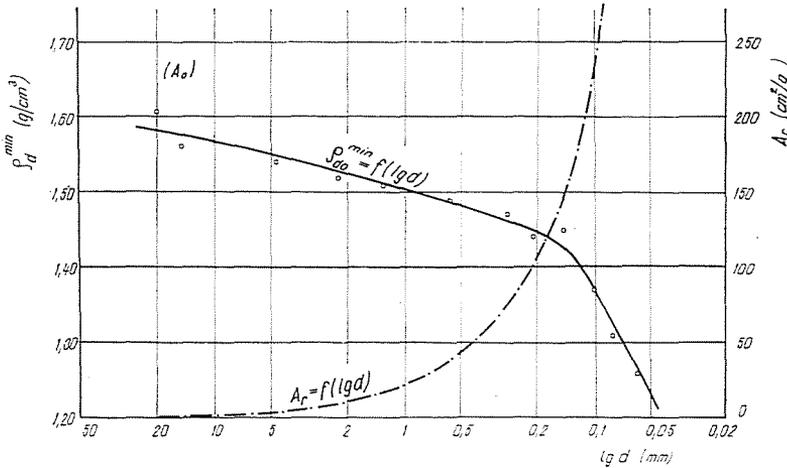
Fig. 6. Specific surface and density of components vs. grain size
