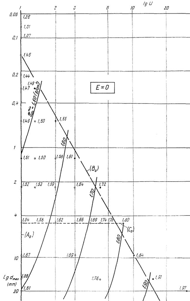
Fig. 5. Poured bulk densities of granular mixes
