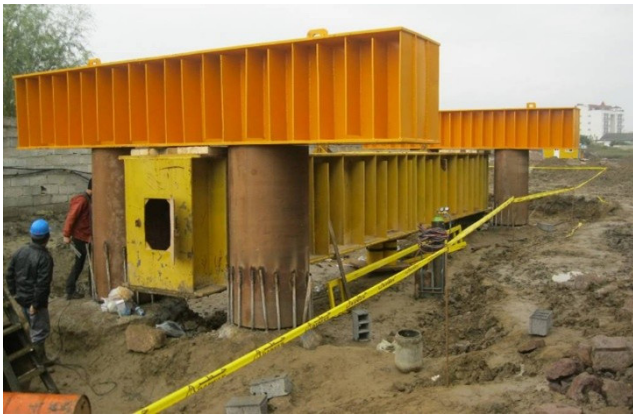
Fig. 8 Field implementation of the Pile Load Test conducted in this study
