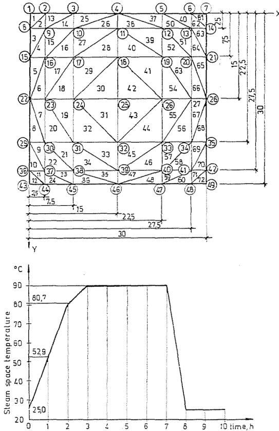
Fig. 6. Division and steam-curing diagram used for testing the effect of material characteristics
