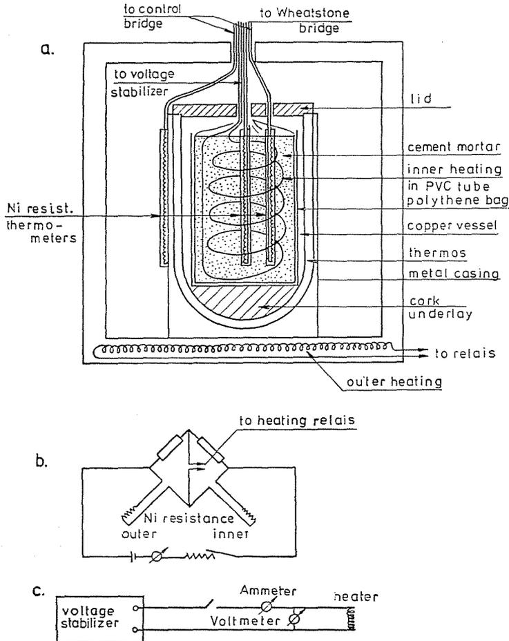
Fig. 7. Sketch of the testing equipment for measuring cement hydration heat and circuit diagram, a) Testing equipment; b) Control bridge of outer heating; c) Control circuit diagram
