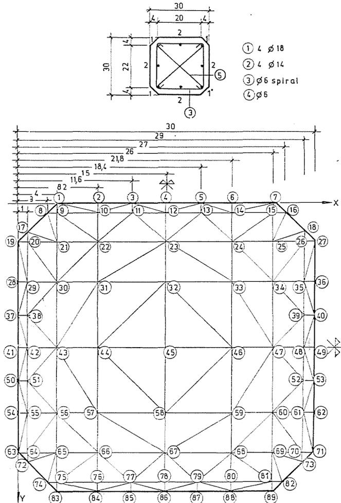
Fig. 9. Reinforcement in column NC-80 and triangle division used for calculating the thermal stresses
