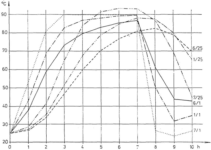
Fig. 4. Concrete temperature development in steam-curing for different heat transfer coefficients (1.  $\alpha = 20 \text{ kcal/m}^2 \text{ h } ^\circ\text{C}$ ; 6.  $\alpha = 10 \text{ kcal/m}^2 \text{ h } ^\circ\text{C}$ ; 7.  $\alpha = 200 \text{ kcal/m}^2 \text{ h } ^\circ\text{C}$ ) at the external corner point of the beam (point No. 1) and in the beam centre (point No. 25)
