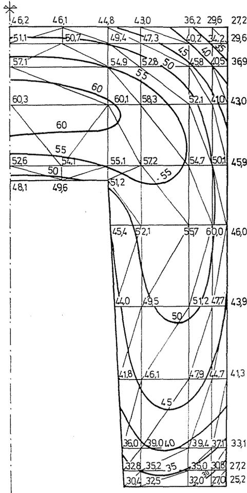
Fig. 12. Isotherms of the temperature field in the cross-section of column Y 46 A, 90 min after taken out of the steam-curing chamber
