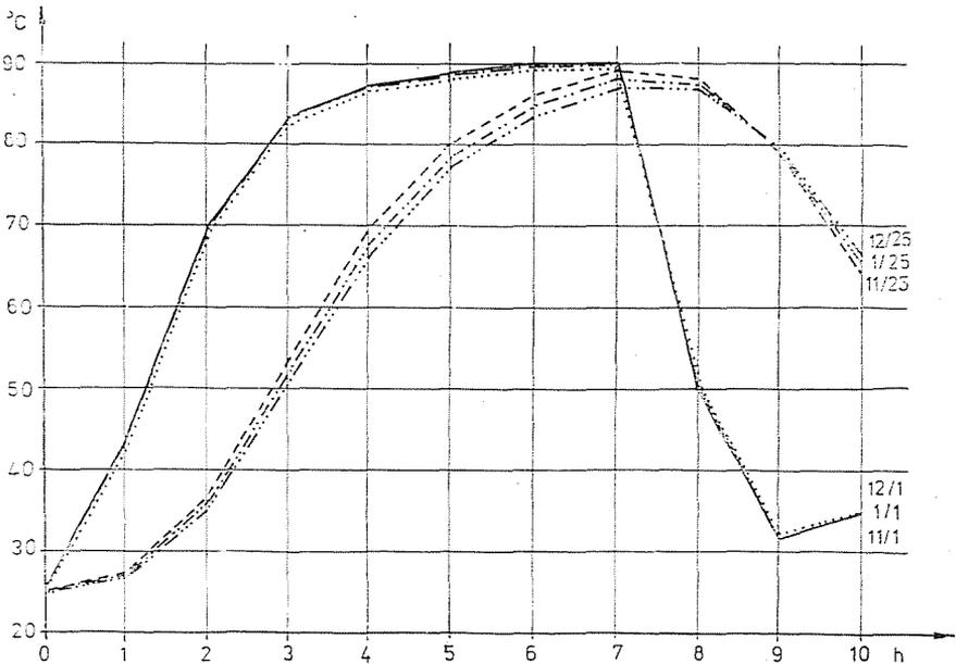
Fig. 5. Development of temperature in steam-curing for different concrete densities (1.  $\gamma = 2400 \text{ kg/m}^3$ ; 11.  $\gamma = 2300 \text{ kg/m}^3$ ; 12.  $\gamma = 2500 \text{ kg/m}^3$ ) at the corner point of the beam (point No. 1) and in the beam centre (point No. 25)
