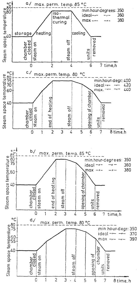
Fig. 1. Steam-curing diagrams used at present in the factory for: a) Beam F (cement C 500, hour/degrees: 360); b) Precast hall units; column, roof slab EP 12, for 12 m main truss beam and reinforced columns (cement C 500, hour/degrees: 360); c) Beam E (cement C 500, hour/degrees: 420); d) Floor units PK. PS (cements C 500, C 600; hour/degrees: 370)
