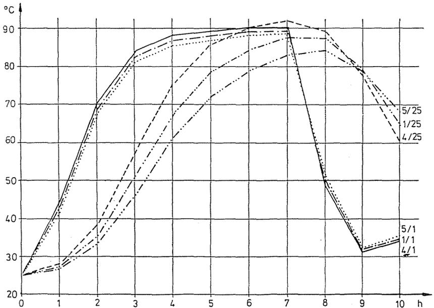
Fig. 3. Concrete temperature development in steam-curing for different specific heat values (1.  $c_b = 0.23$  kcal/kg °C; 4.  $c_b = 0.19$  kcal/kg °C; 5.  $c_b = 0.27$  kcal/kg °C) at the corner point of the beam (point No. 1) and in the beam centre (point No. 25)
