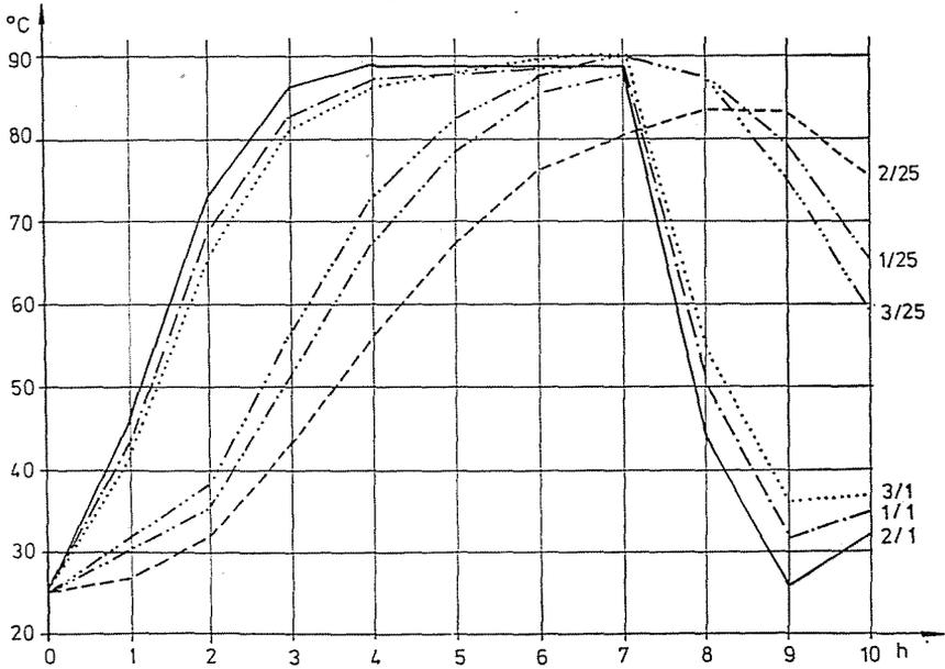
Fig. 2. Concrete temperature development in steam-curing for different heat conductivities (1.  $\lambda = 1.8$  kcal/m h °C, 2.  $\lambda = 0.9$  kcal/m h °C, 3.  $\lambda = 2.7$  kcal/m h °C), on the beam surface (point No. 1) and in the centre of the beam (point No. 25)
