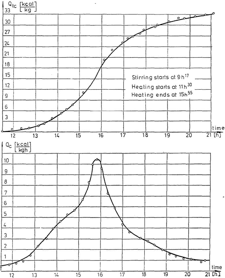
Fig. 8. Development and rate of hydration development of Portland cement C 500 DCM throughout steam-curing in test 4. (Initial temperature 25.18 °C, final temperature 73.4 °C)
