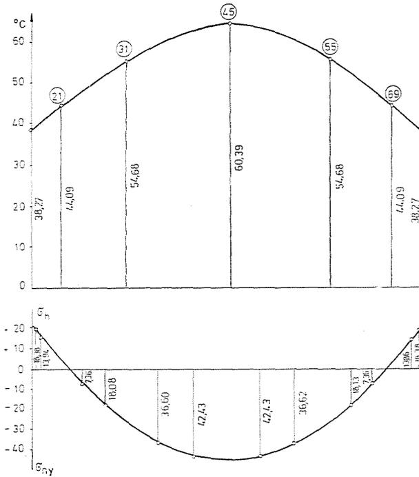
Fig. 10. Temperature and stress distribution in the diagonal section of the column NC-80 90 min after taken out of the steam-curing chamber
