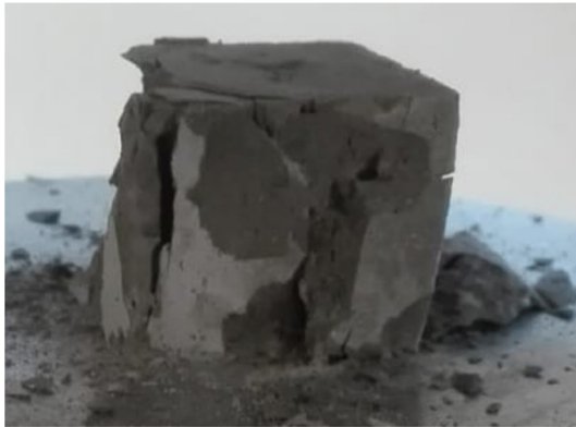
Fig. 7 Compressive strength test for 25%, MA CDW 60 based binder
