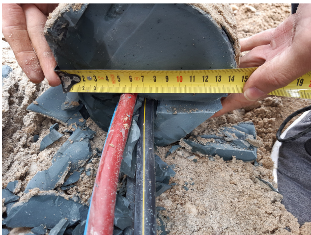
Fig. 4 Diameter of excavated anchor at Pillar project
