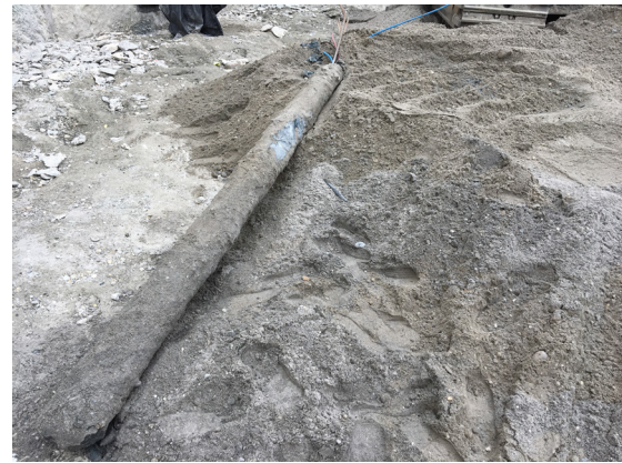
Fig. 1 Excavated anchor body at Taksony Street project
