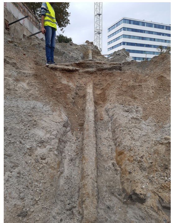
Fig. 2 excavated anchor body showing irregular shape masses at Pillar project
