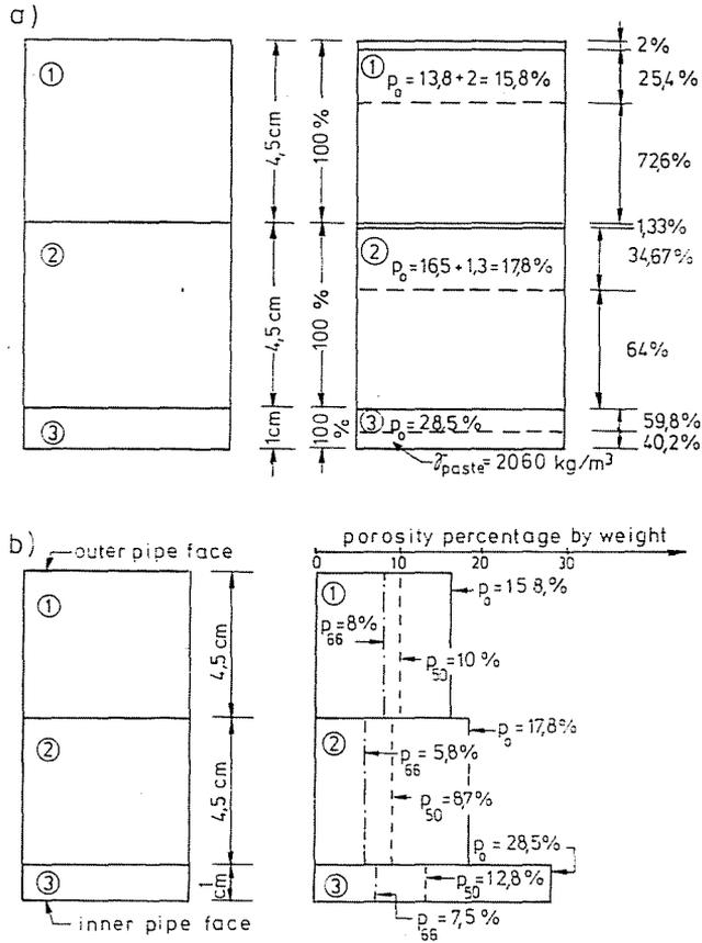
Fig. 1. Structural model for a 3-layered inhomogeneous concrete unit (e.g. concrete pipe)
