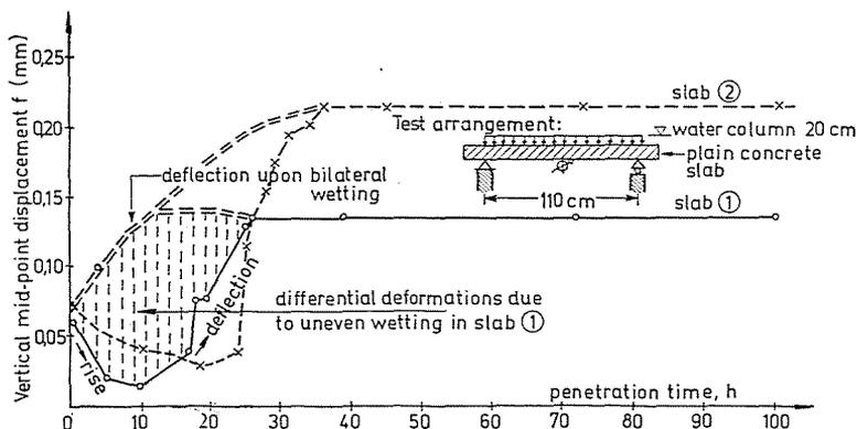
Fig. 3. Effect of one-side wetting on the vertical displacement of the middle cross-section of a self-supporting plain concrete slab
