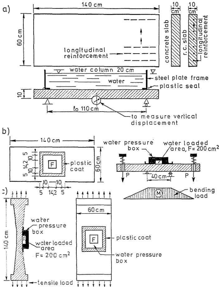
Fig. 2. Concrete specimens and test arrangement. a) Low water pressure (unilateral wetting); b) Combined effect of bending load and water pressure; c) Combined effect of tensile load and water pressure (10 cm unit thickness at the spot under water pressure)
