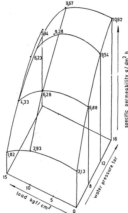
Fig. 8. Combined effect of flexural load and water pressure at the compressed side on the specific value of permeability of a r. c. slab
