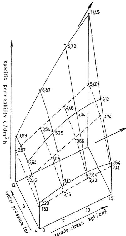
Fig. 7. Combined effect of tensile load and water pressure on the specific value of permeability of a r. c. slab. Legend: - - - - Concrete grade B 450; ————— Concrete grade B 280
