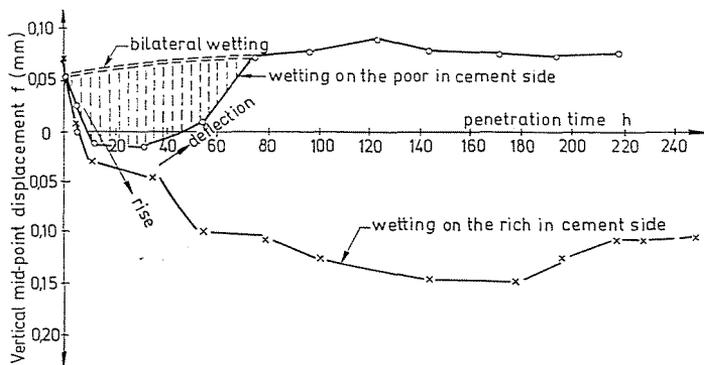
Fig. 6. Vertical displacement of the middle cross-section of a layered inhomogeneous concrete slab under the effect of one-side wetting (three-layered model as shown in Fig. 1)
