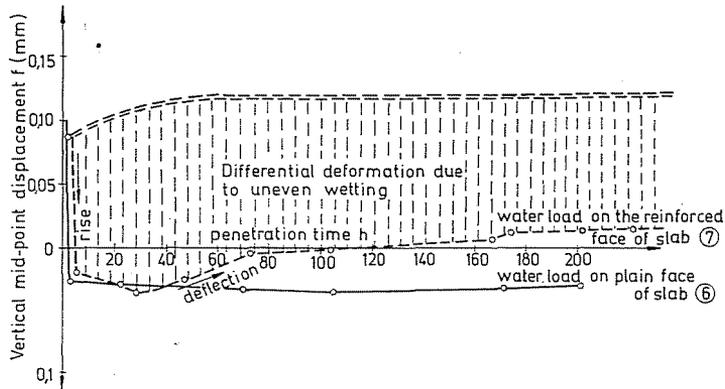
Fig. 5. Effect of one-side wetting on the vertical displacement of the middle cross-section of a self-supporting concrete slab with 10 mm reinforcement
