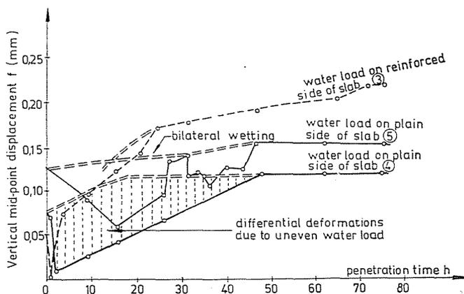
Fig. 4. Effect of one-side wetting on the vertical displacement of the middle cross-section of a self-supporting concrete slab with 14 mm reinforcement
