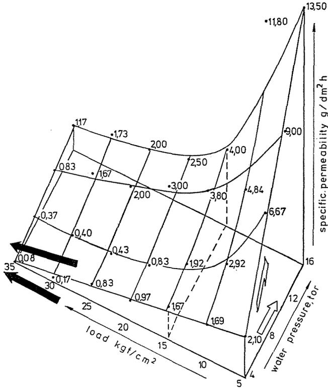
Fig. 9. Combined effect of flexural load and water pressure at the tensile side on the specific value of permeability of a r. c. slab
