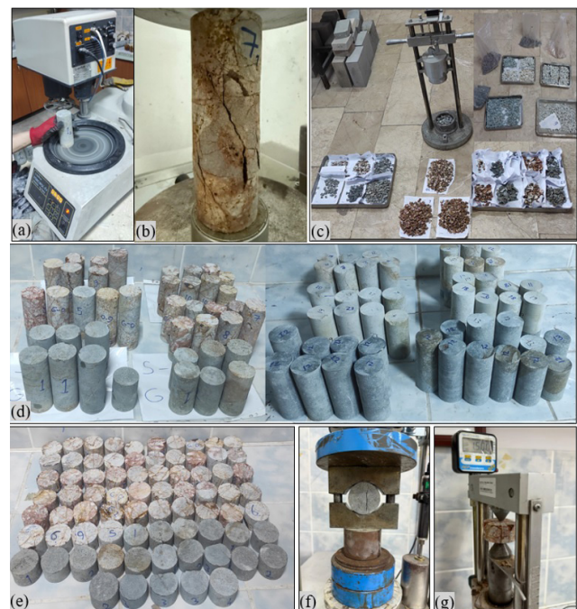
Fig. 4 Images from experimental studies: (a) core grinding, (b) appearance after the UCS test, (c) AIV test, (d) representative dacite cores, (e) disc samples, (f) BTS test, and (g) PLI test
