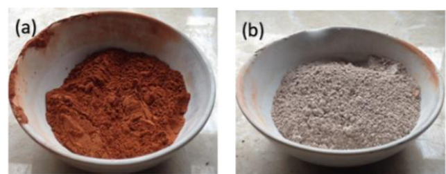
Fig. 1 Waste materials used in the study: (a) Brick tile powder; (b) Ceramic tile powder
