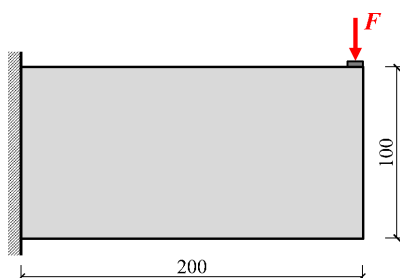
Fig. 5 Illustration of the planar cantilever beam problem [18] (units: mm)
