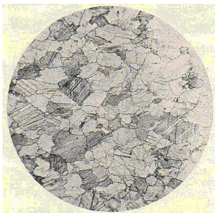
**Fig. 7.** The microscopic picture of the marble after 9% permanent deformation and after changing under a 2500 atm or 253 MPa pressure (magnification 50X) [8]
