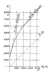
Fig. 15. Relationship between the main stresses ("állandó" means constant) according to Kármán [8]
