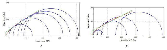
Fig. 14. The recalculated limit lines of the (A) marble and (B) sandstone (the overlaid envelopes: Mohr-Coulomb with green and Hoek-Brown with red color)
