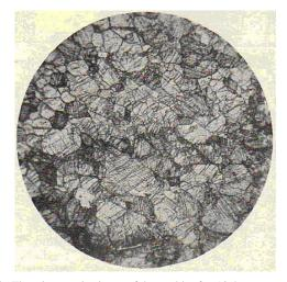
**Fig. 9.** The microscopic picture of the marble after 13% permanent fore and aft changing under an 500 atm, or 50,7 MPa pressure (magnification 50X) [8]
