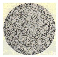
**Fig. 6.** The microscopic picture of the marble before deformation (magnification 50X) [8]
