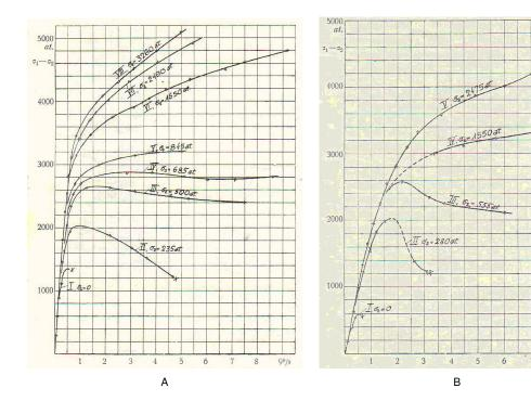
Fig. 3. The effective stress vs. deformation of (A) Carrara marble and (B) Mutenberg sandstone rock samples in case of different confining pressures. (1 atm = 0.101325 MPa) [8]
