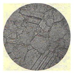
**Fig. 10.** The microscopic picture of the marble before deformation (magnification 175X) [8]
