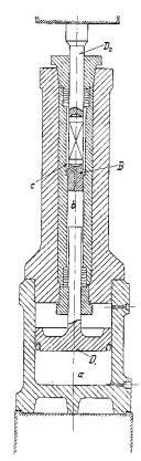
Fig. 1. "The Bomb", the triaxial cell of Kármán [8]
