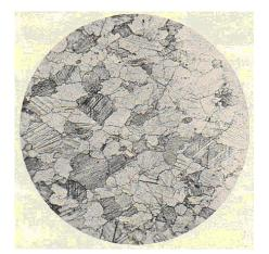
**Fig. 7.** The microscopic picture of the marble after 9% permanent foreandaft changing under a 2500 atm or 253 MPa pressure (magnification 50X) [8]
