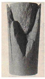
Fig. 5. Cracking of a sandstone sample after a normal uniaxial strength testing [8]
