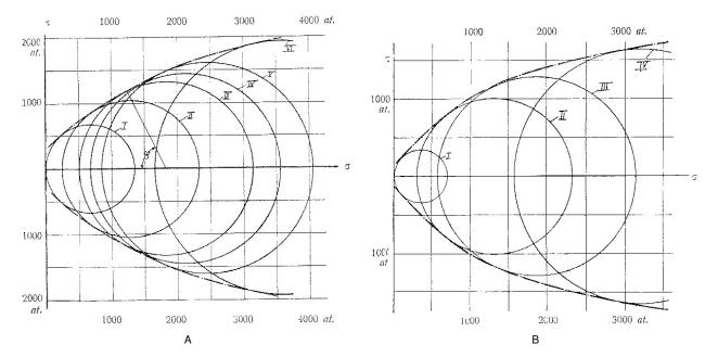
Fig. 13. The limit line of the (A) marble and (B) sandstone using the Mohr theory, according to Kármán [8]
