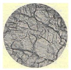
**Fig. 12.** The microscopic picture of the intergranular deformation (magnification 175X) [8]
