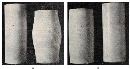
Fig. 4. The original (left on A, and right on B) and due to low (A) and high (B) confining pressure deformed marble sample (right on A, and left on B) [8]
