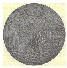
**Fig. 11.** The typical view of intragranular deformation (magnification 175X) [8]
