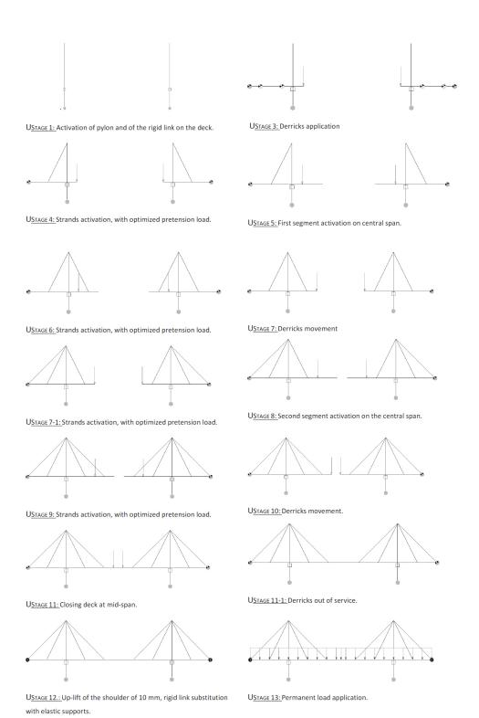
Fig. 6. Construction phase, lateral cantilever method
