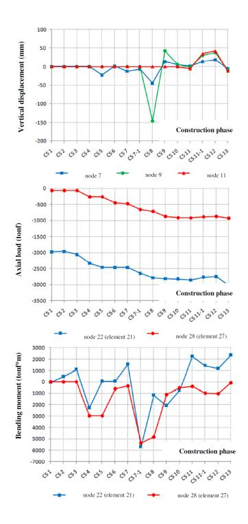
Fig. 16. Vertical displacement variation in the central span, axle load variation in the pylon, bending moment variation in the pylon (NLSA\_nlg) ( $1 \cot 10 \text{ kN}$ )
