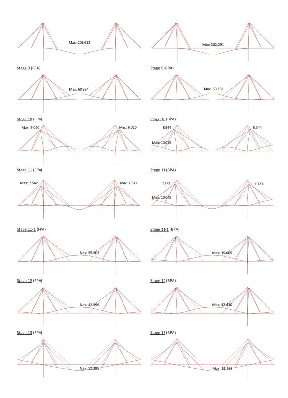
**Fig. 20.** Structure configuration during the partial cantilevered construction phases, measures in [mm]: comparison between back (BPA) and forward analysis (FPA) (Stages 8-13)
