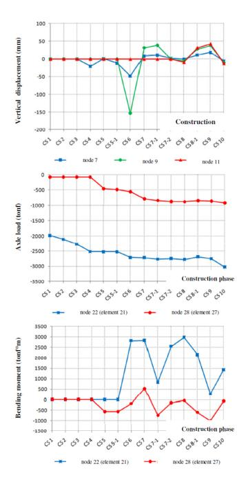
Fig. 24. Vertical displacement variation of the lateral span, axle load variation in cables, bending moment variation in the pylon (NLSA\_nlg) (1 tonf=10 kN)
