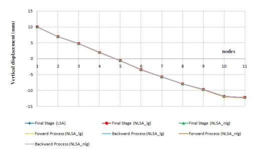
Fig. 12. Vertical displacement in the control points of the girder, partial cantilever construction mode
