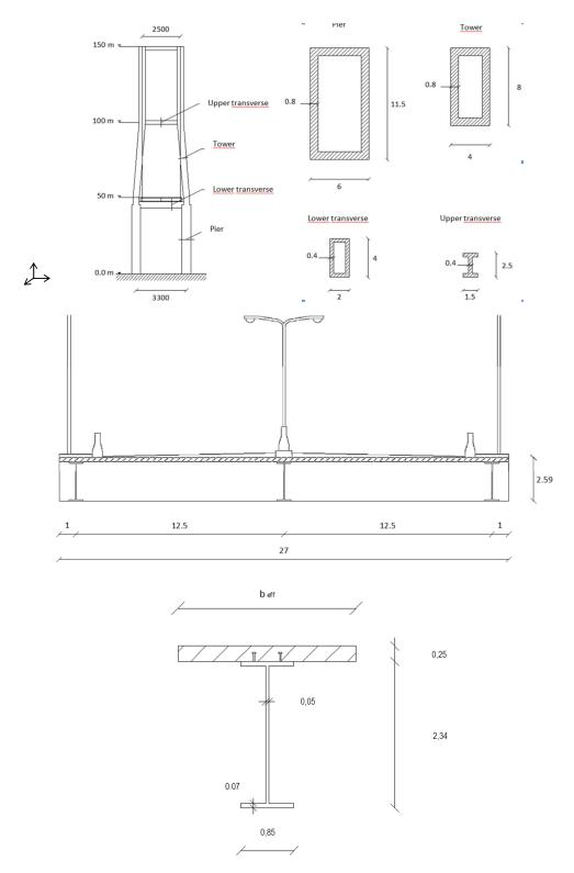
Fig. 2. Bridge details (unit in metre)
