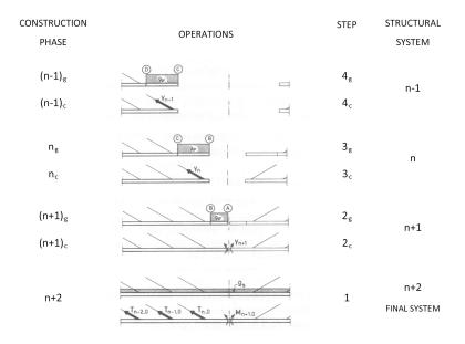
Fig. 7. Moving load due to the movement of the derric
