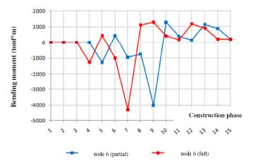
Fig. 30. Bending moment variation in the central span (NLSA\_nlg) (1 tonf=10 kN)  $\,$
