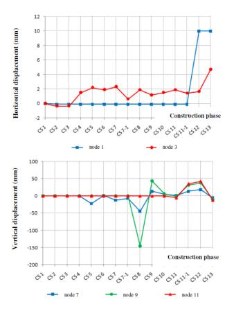
Figure 22 highlights the configurations during the construction process, with a forward analysis and the corresponding displacements. In the following are presented the results obtained in relation to the axle load on cables, the horizontal displacement at the top of the pylon, the vertical displacement of the girders, and the axial and bending forces in some sections of the pylon and the girder (Figs. 23-25).
