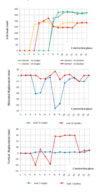
Fig. 28. Axle load variation in cables, Horizontal displacement variation in the pylon, Vertical displacement variation in the lateral span (NLSA\_nlg) (1  $tonf=10\ kN$ )
