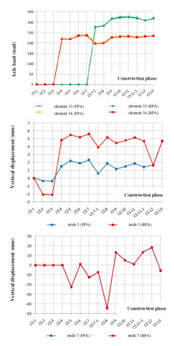
Fig. 21. Axle load variation in cables, node 3 variation of the vertical displacement, node 7 variation of the vertical displacement (NLSA\_nlg) (1 tonf=10 kN)
