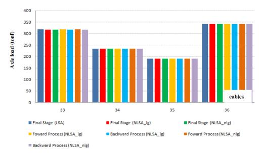
Fig. 11. Axle load in cables, partial cantilever construction mode (1 tonf=10 kN)
