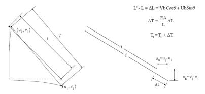
Fig. 8. Lack of Fit Force calculation in a cable
