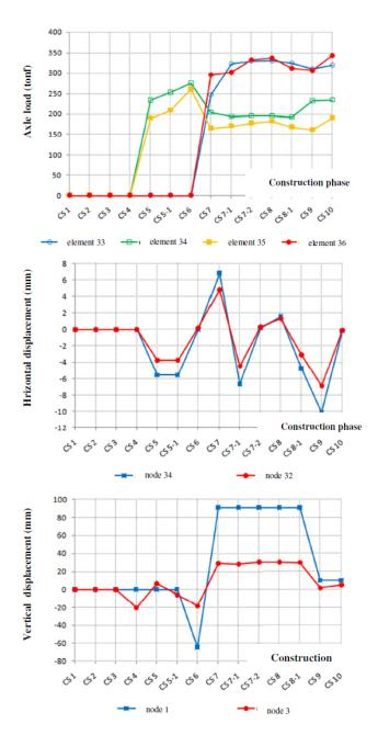
**Fig. 23.** Axle load variation in cables, horizontal displacement variation of tonf=10 kN; the pylon, vertical displacement variation of the lateral span (NLSA\_nlg) (1
