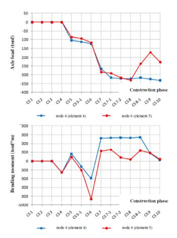
$\textbf{Fig. 25.} \ \ \, \text{Axle load variation in the girder, bending moment variation in the girder (NLSA\_nlg) (1 tonf=10 \ kN)}$
