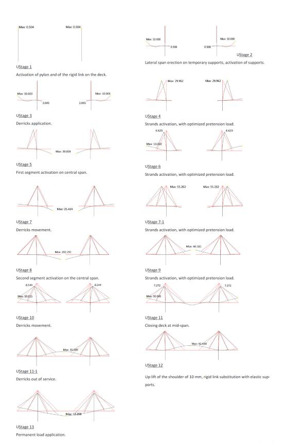
Fig. 14. Structure configuration during the partial cantilevered construction phases (BPA)
