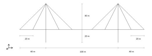
Fig. 1. Overall bridge layout (unit in metre)
