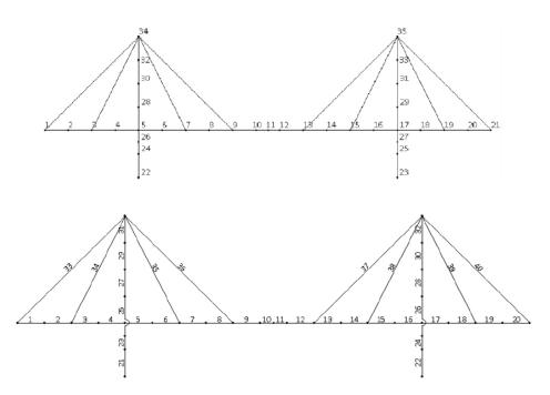
$\textbf{Fig. 10.} \ \ \textbf{FEM reference for the model, nodes and elements numerations}$
