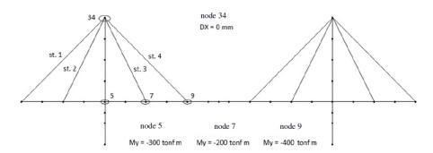
Fig. 4. Imposed conditions on the bridge structure
