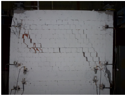
(a) Typical cracks on specimen
