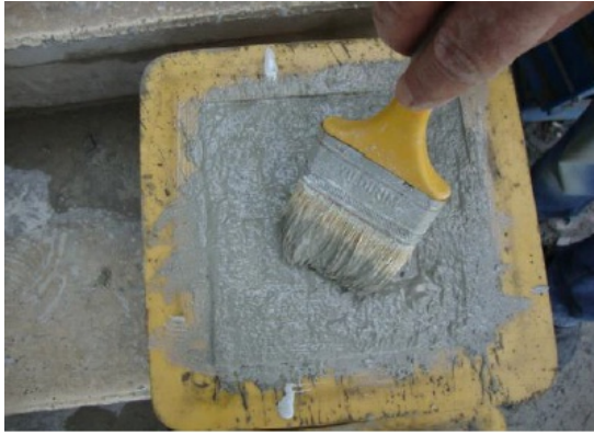
a) Curing material application on a specimen
