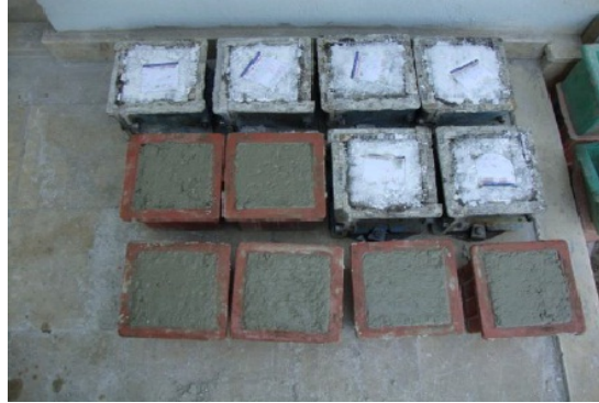
b) After the application of curing material
