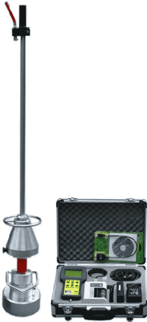
Fig. 1. The B&C small-plate device
