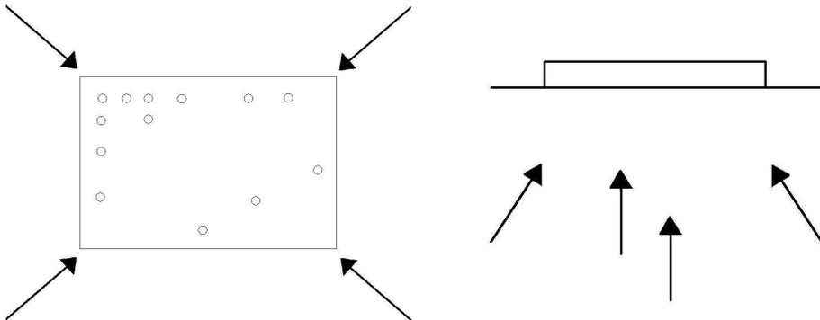
*Fig. 6.* Locations of taking photographs Manhattan-type test-field
