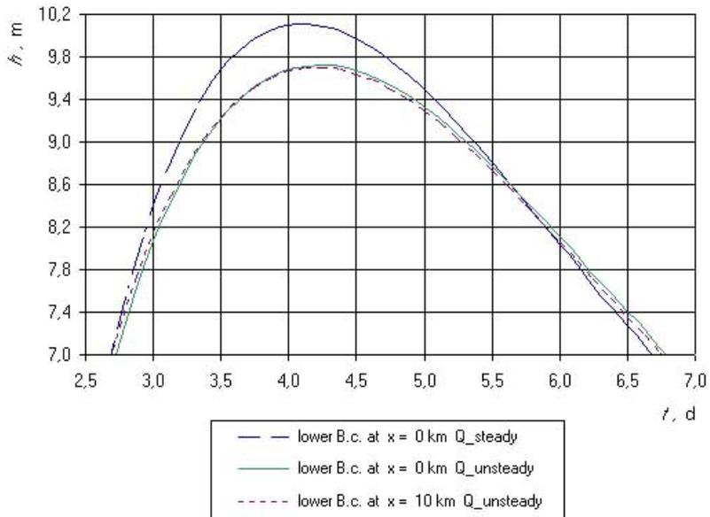
Fig. 5. The  $h = h(t)$  hydrographs at the  $x = 10$  km lower boundary section
