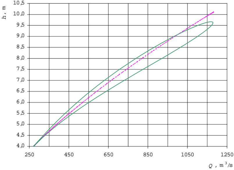
Fig. 2. The steady rating curve and unsteady loop curve at the  $x = 0$  km section
