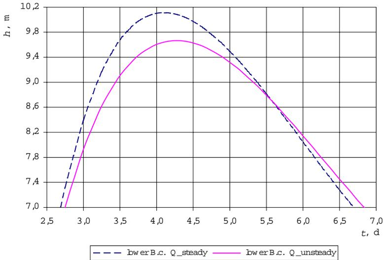
Fig. 3. The  $h = h(t)$  hydrographs at the  $x = 0$  km lower boundary section
