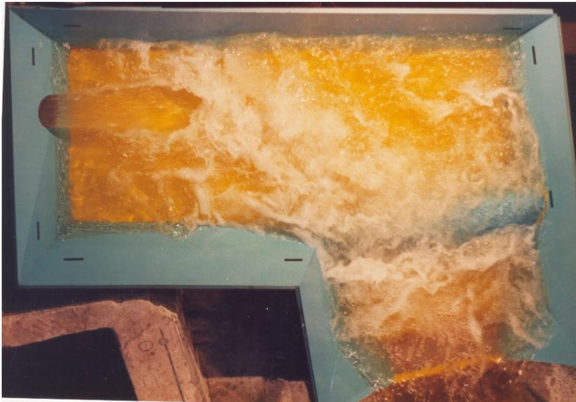
*Picture 2.* Proposed variant of the stilling basin system in 1:50 scale model with the design discharge of  $810 \text{ m}^3/\text{s}$
