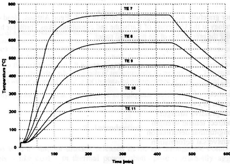
Fig. 10. Temperature distribution by the different thermoelements in the Postaer sandstone
