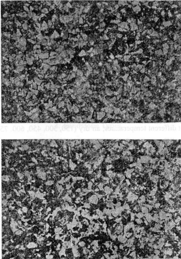
*Fig. 1.* Thin sections analyses by polarising microscope. a) Rohrschacher sandstone, at 22°C; b) Rohrschacher sandstone at 900°C
