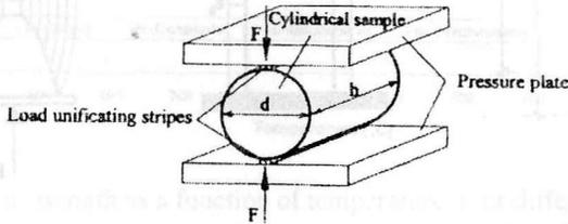
Fig. 4. Test configuration of indirect tensile strength measurements (ALFES – SCHIESSL, 1994)
