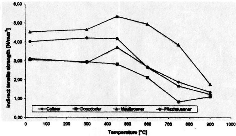
Fig. 5. Indirect tensile strength of four different sandstone types as a function of temperature
