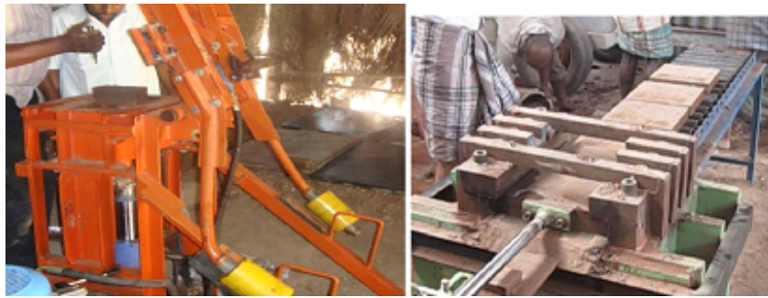
Fig. 1. Manufacturing of Solid , Hollow block in Auram 3000 and Modified solid block in Auram 4000
