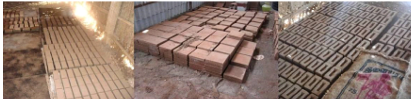
Fig. 2. Solid, Modified Solid and Hollow compresses stabilised Earth blocks
