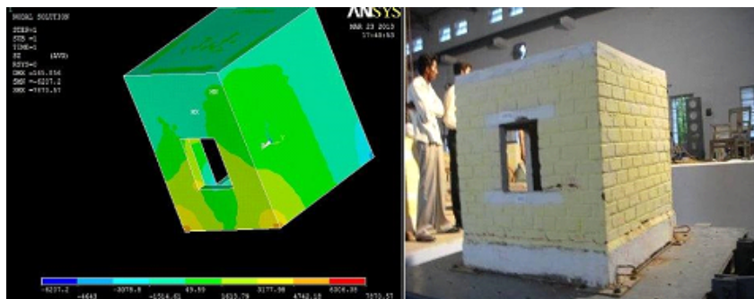
Fig. 23. S1 Model at 0.2689 g – crack pattern
