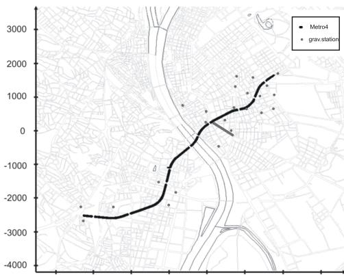
Fig. 2. The tunnel (solid black line interrupted at the stations) and the gravimetric points (grey stars) with main structures of Budapest in the background. The axis are local stereographic coordinates in m.
