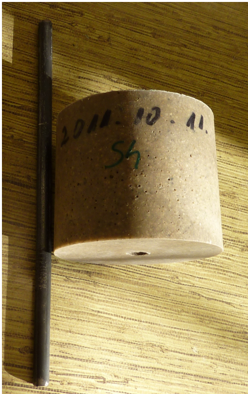
Fig. 3. Specimen destroyed by the pull-out of the reinforcing rebar
