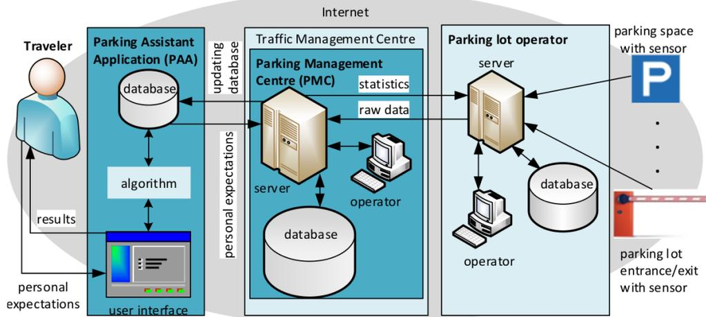
Fig. 4. Structural model of PAS (source: own)
