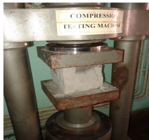
Fig. 3. Compressive strength test by CTM
