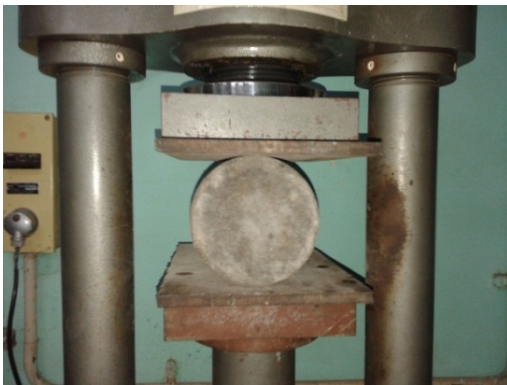
Fig. 8. Split tensile strength test
