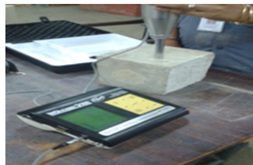
Fig. 13. Compressive strength test by RH
