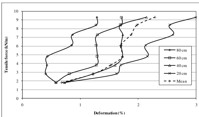
Fig. 8. Maximum tensile force vs GCL strain (80 cm curve not considered in mean curve)
