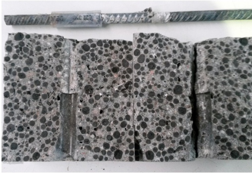
Fig. 7. Specimen (LWFC-0-1) overview after Pull-out test
