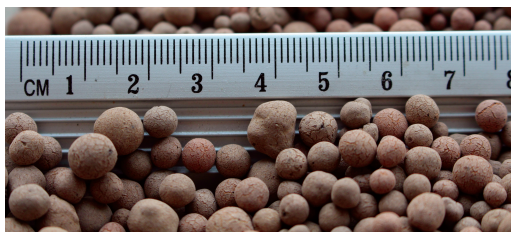
Fig. 1. Expanded clay used as coarse aggregate
