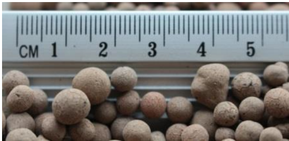
Fig. 1 Expanded clay used as coarse aggregate
