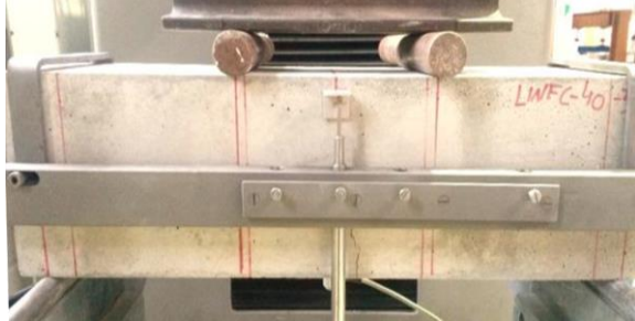
Fig. 6 Failure crack propagation in maximum moment area during four point bending test
