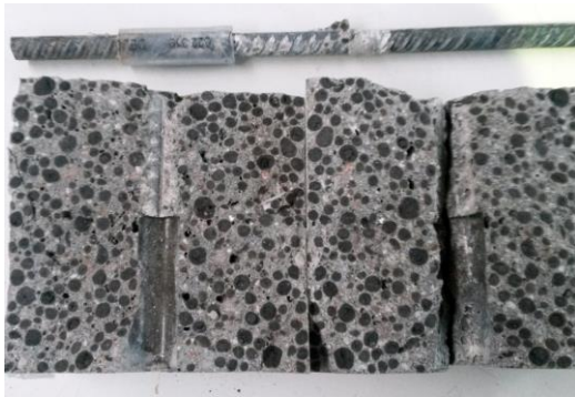
Fig. 7 Specimen (LWFC-0-1) overview after Pull-out test
