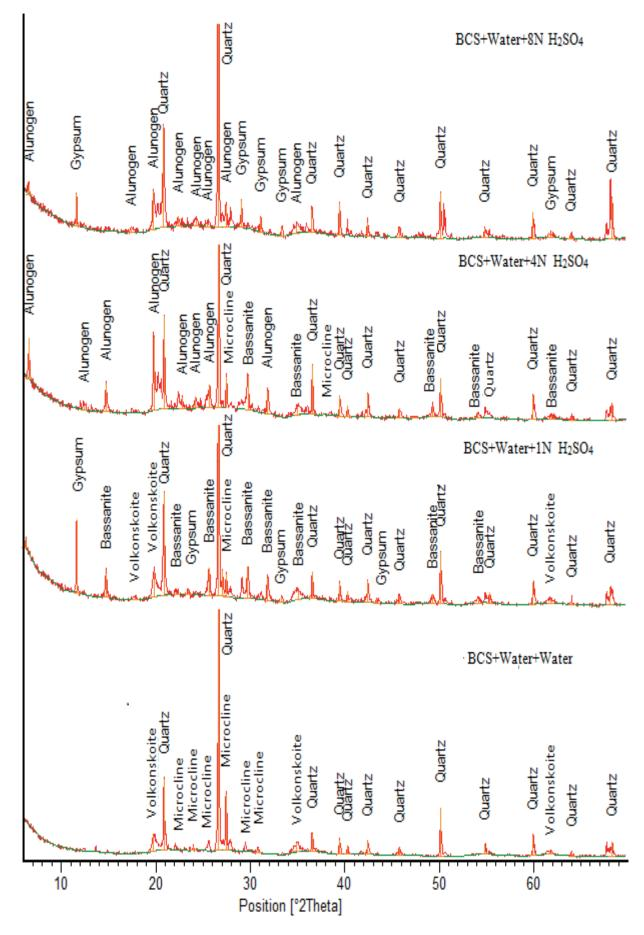
Fig. 6 X-ray diffraction patterns of black cotton soil after free swell with Water and H<sub>2</sub>SO<sub>4</sub> solutions
