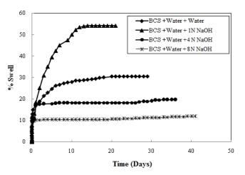
Fig. 2 Influence of pore fluids water and NaOH solutions on free swell behaviour of black cotton soil
