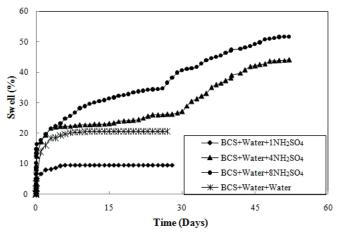
Fig. 5 Influence of pore fluids water and  $H_2SO_4$  solutions on free swell behaviour of black cotton soil
