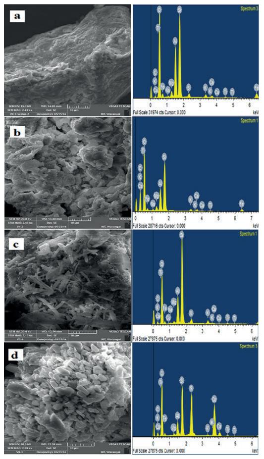
Fig. 7 Scanning electron microscopy and Energy dispersive analysis of X-ray images of black cotton soil after free swell with (a) Water (b)  $1N H_2SO_4$  (c)  $4N H_2SO_4$  and (d)  $8N H_2SO_4$
