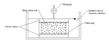
Fig. 1 Free swell test set up with black cotton soil in Teflon made ring
