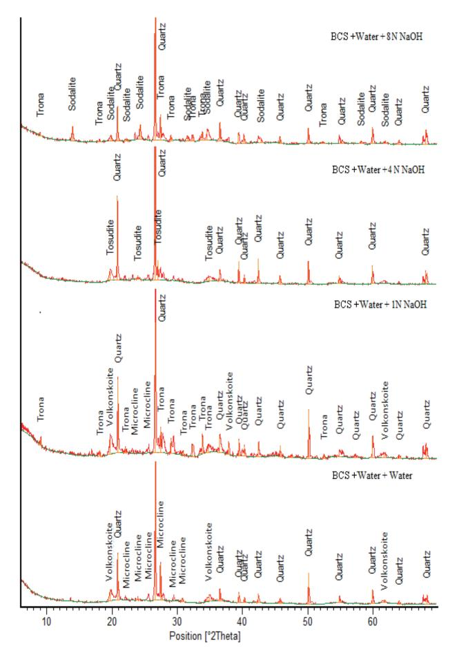
Fig. 3 X-ray diffraction patterns of black cotton soil after free swell with Water and NaOH solutions
