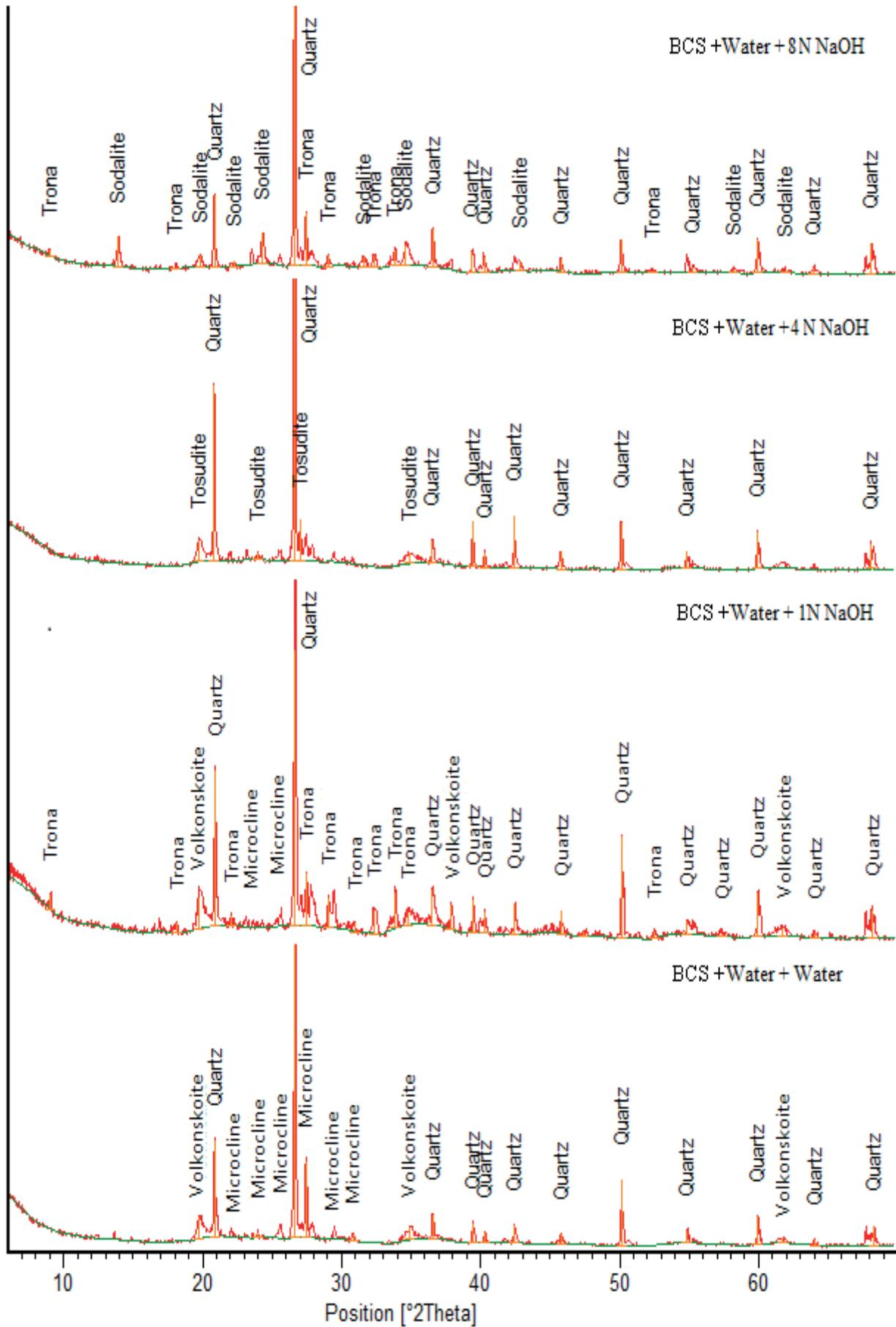
Fig. 3 X-ray diffraction patterns of black cotton soil after free swell with Water and NaOH solutions
