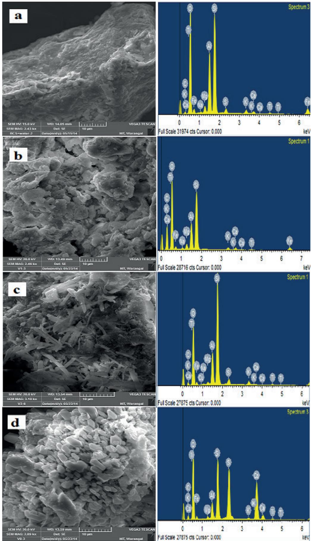
Fig. 7 Scanning electron microscopy and Energy dispersive analysis of X-ray images of black cotton soil after free swell with (a) Water (b) 1N H<sub>2</sub>SO<sub>4</sub> (c) 4N H<sub>2</sub>SO<sub>4</sub> and (d) 8N H<sub>2</sub>SO<sub>4</sub>
