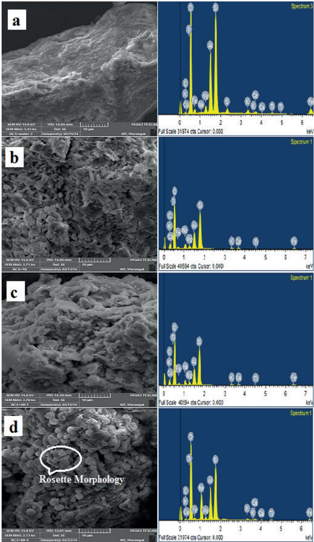
Fig. 4 Scanning electron microscopy and Energy dispersive analysis of X-ray images of black cotton soil after free swell with (a) Water (b) 1N NaOH (c) 4N NaOH and (d) 8N NaOH
