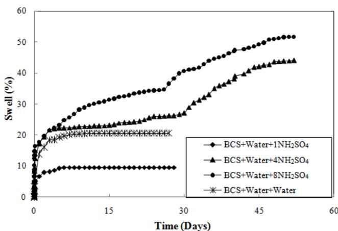
Fig. 5 Influence of pore fluids water and H<sub>2</sub>SO<sub>4</sub> solutions on free swell behaviour of black cotton soil
