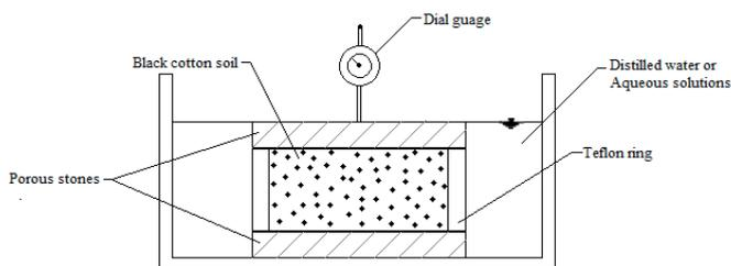
Fig. 1 Free swell test set up with black cotton soil in Teflon made ring
