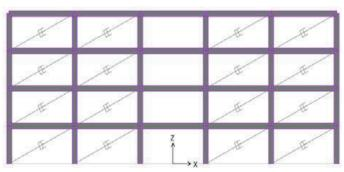
(e) 80% of bays of structures equipped with damper devicesFig.7 Structures with different damper assignments
