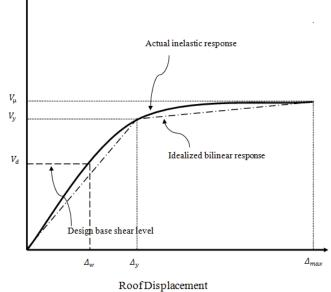
Fig. 1 Idealization of the inelastic response of a structure
