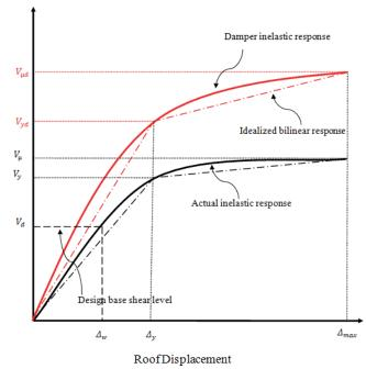
Fig.2 Idealization of the inelastic response of structures with and without damper devices
