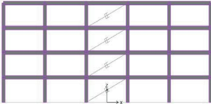
(b) 20% of bays of structures equipped with damper devices
