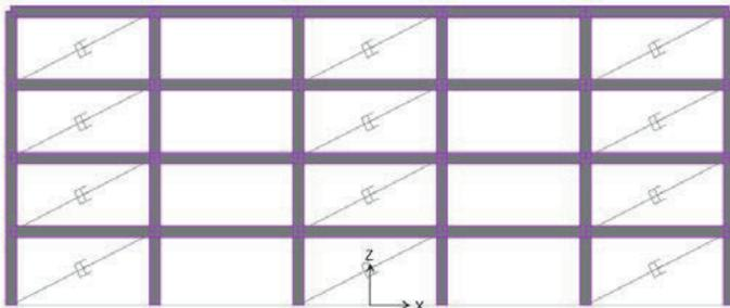
(d) 60% of bays of structures equipped with damper devices
