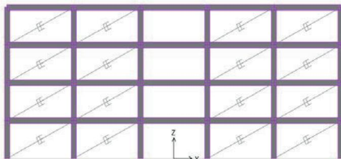
(e) 80% of bays of structures equipped with damper devices
