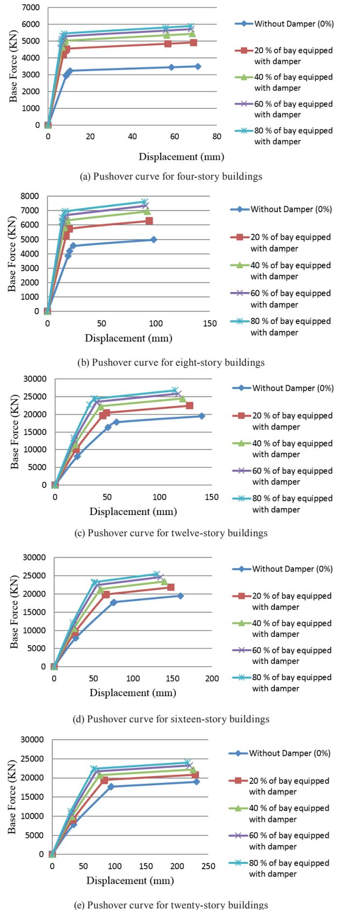
Fig. 8 Pushover curve for viscous damper with  $C = 0.2568533 \text{ (kN}\cdot\text{s/mm)}$
