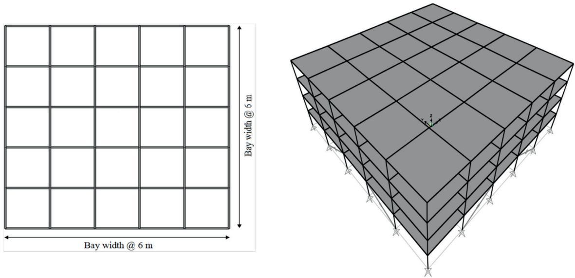
Fig.4 Structural arrangement of buildings in the plan
