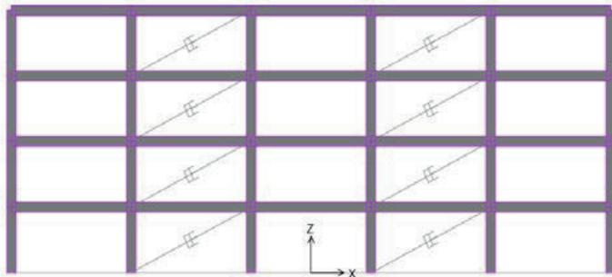
(c) 40% of bays of structures equipped with damper devices
