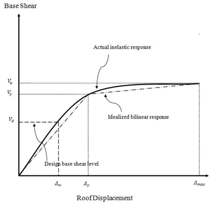
Fig. 1 Idealization of the inelastic response of a structure
