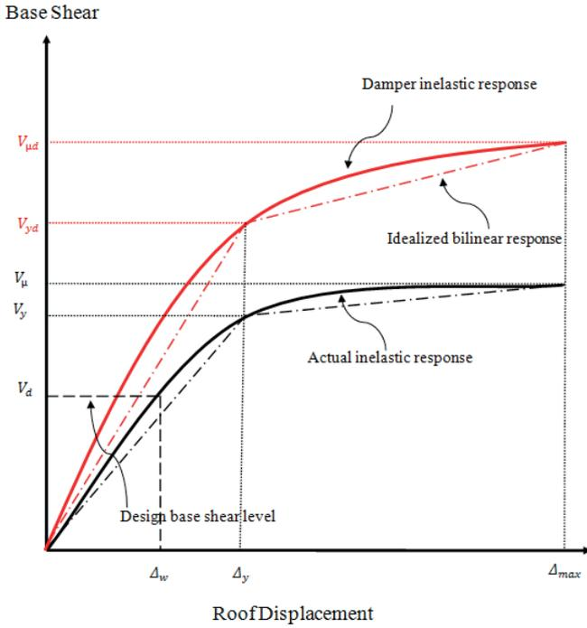
Fig.2 Idealization of the inelastic response of structures with and without damper devices
