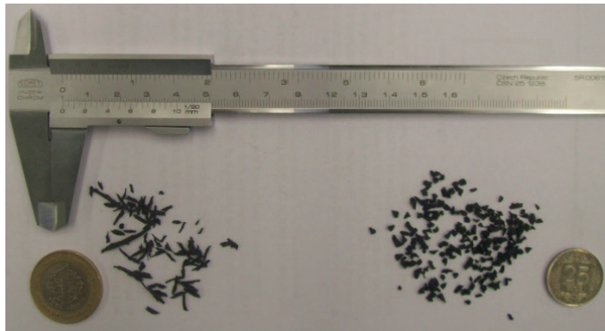
Fig. 1 Tire buffings and tire crumbs samples used in the experimental studies
