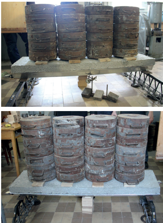
Fig. 7 Test specimen – the polystyrene concrete slab with profiled steel sheeting
