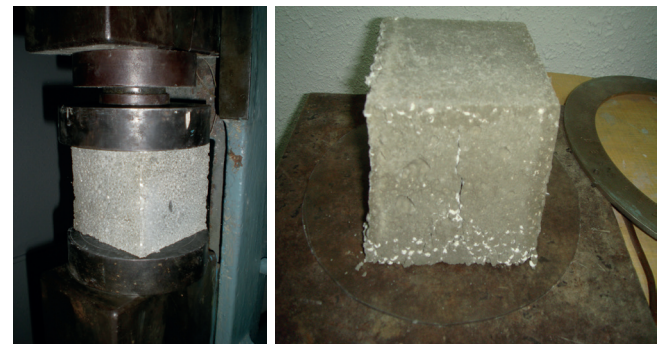
Fig. 4 The strength test of the polystyrene concrete cubs
