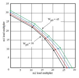
Fig. 8 Safe loading domain for plastic limit design
