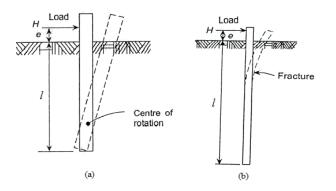
Fig. 1 Failure mechanisms of pile under horizontal load: (a) short rigid pile, (b) long pile
