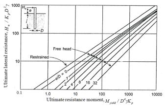
Fig. 2 Design chart for long piles in cohesionless soil
