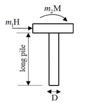
Fig. 9 Loads on the fixed-head pile
