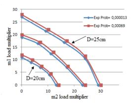
Fig. 7 Safe loading domain for plastic limit design
