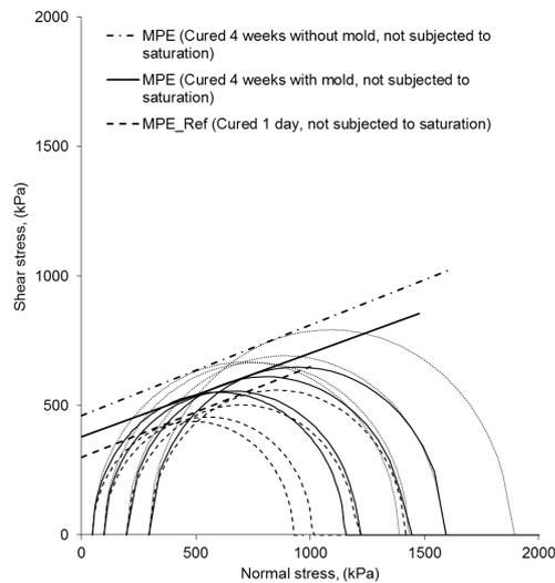
**Fig. 8.** Mohr circles and Mohr-Coulomb failure envelopes of samples compacted at MPE level (effect of keeping in mold)
