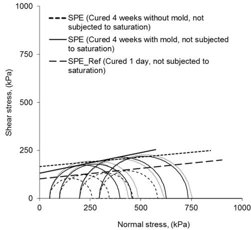
**Fig. 7.** Mohr circles and Mohr-Coulomb failure envelopes of samples compacted at SPE level (effect of keeping in mold)
