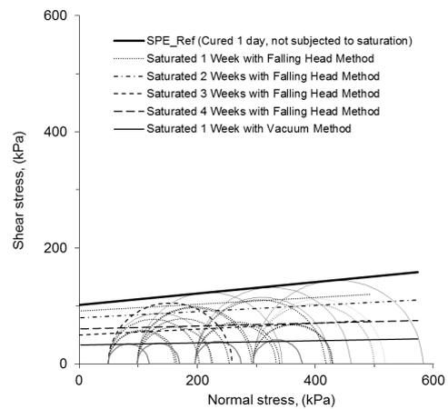
**Fig. 9.** Mohr circles and Mohr-Coulomb failure envelopes of samples compacted at SPE level (Influence saturation process)
