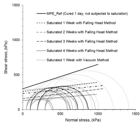
**Fig. 10.** Mohr circles and Mohr-Coulomb failure envelopes of samples compacted at MPE level (Influence saturation process)
