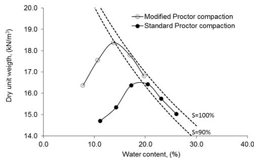
Fig. 2. Standard and Modified Proctor compaction curves of the soil
