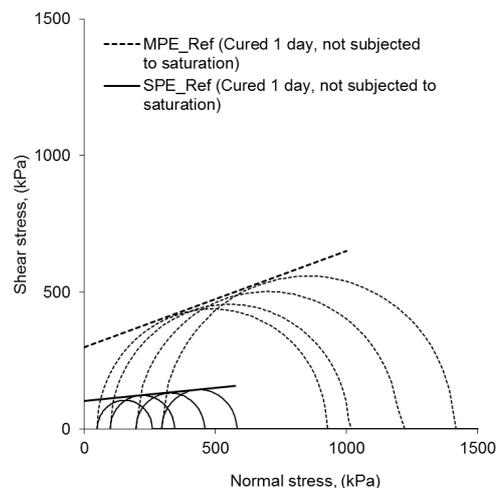
Fig. 6. Mohr circles and Mohr-Coulomb and failure envelopes of the reference samples (Cured one day and not subjected to any saturation process).
