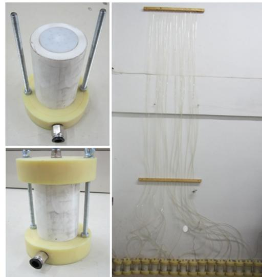
Fig. 4. Falling head saturation method setup (Bahari Kheirjouy, 2014)
