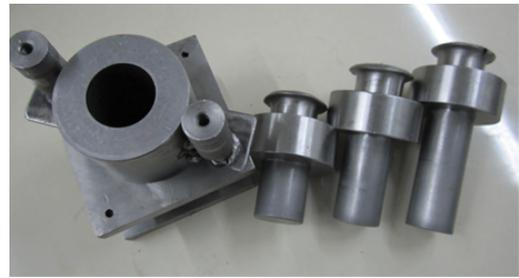
Fig. 3. Triaxial test sample preparation apparatus (Bahari Kheirjouy, 2014)
