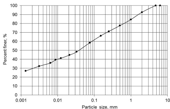
Fig. 1. Particle size distribution curve of the soil used in the study summarizes the consistency limits, specific gravity and soil class according to the Unified Soil Classification System (USCS)
