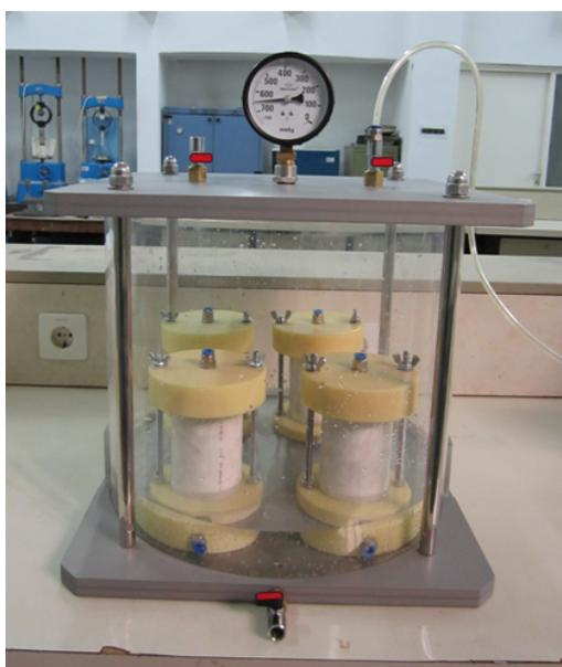
Fig. 5. Vacuum saturation method setup (Bahari Kheirjouy, 2014)
