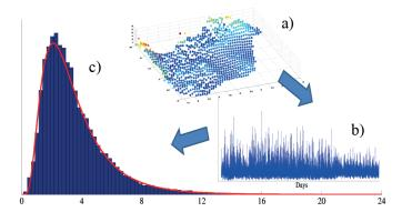
**Fig. 6** Evaluation of the distribution of daily maximum wind speeds: a) EN conforming characteristic wind speeds in Hungary; b) daily maximum wind speeds for 50 years at the selected coordinate; c) fitted distribution
