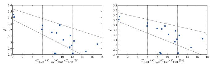
Fig. 10 Optimal safety levels as a function of additional costs comparing to the configurations in Table 8: a)  $\rho = 0.4$ ; b)  $\rho = 0.9$  correlation coefficient
