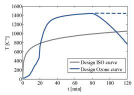
Fig. 3 The difference between ISO and Ozone fire curves
