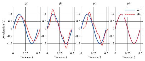
Fig. 2 Type of discrepancies in the shaking table feedbacks, (a) Amplitude and phase errors (b) Spurious harmonics (c) a and b combined (d) Ideal case
