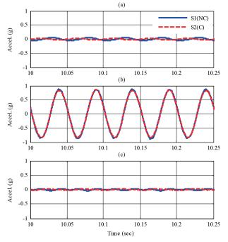
**Fig. 11** Translational accelerations achieved on the CGS shaking table, (a): Longitudinal, (b): Tansversal and (c): Vertical, for sinusoidal tests S1 and S2
