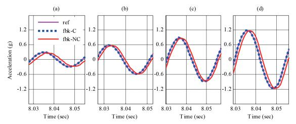
Fig. 5 Shaking table reference (ref) and feedbacks, compensated (fbk-C) and uncompensated (fbk-NC), of harmonic tests at 40 Hz, performed whit peak amplitudes of (a) 0.30; (b) 0.60; (c) 0.90 and (d) 1.20g
