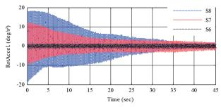
Fig. 15 Roll acceleration feedbacks of the CGS shaking for sinusoidal tests S6, S7 and S8
