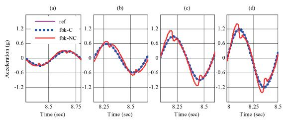
Fig. 3 Shaking table reference (ref) and feedbacks, compensated (fbk-C) and uncompensated (fbk-NC), of harmonic tests at 2 Hz, performed whit peak amplitudes of (a) 0.30; (b) 0.60; (c) 0.90 and (d) 1.20g
