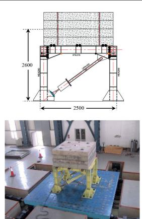
Fig. 10 View of the test specimen
