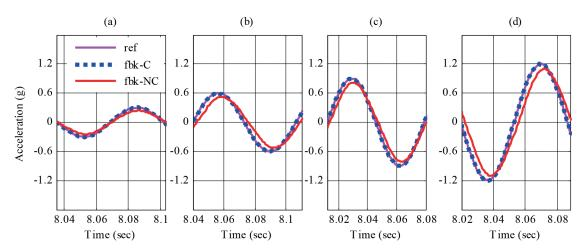
Fig. 4 Shaking table reference (ref) and feedbacks, compensated (fbk-C) and uncompensated (fbk-NC), of harmonic tests at 15 Hz, performed whit peak amplitudes of (a) 0.30; (b) 0.60; (c) 0.90 and (d) 1.20g
