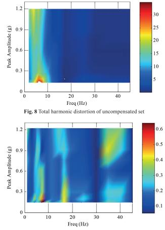
Fig. 9 Total harmonic distortion of compensated tests set
