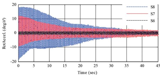
**Fig. 15** Roll acceleration feedbacks of the CGS shaking for sinusoidal tests S6, S7 and S8
