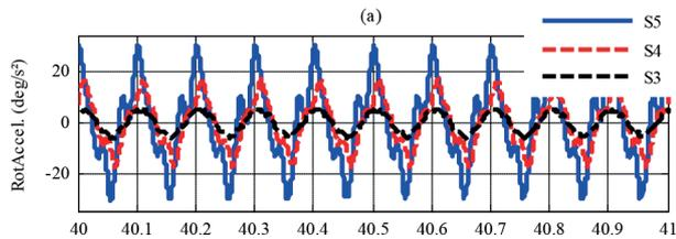
**Fig. 13** Roll acceleration feedbacks of the CGS shaking for sinusoidal tests S3, S4 and S5
