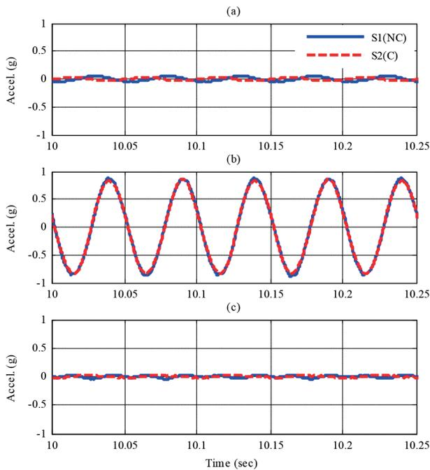
**Fig. 11** Translational accelerations achieved on the CGS shaking table, (a): Longitudinal, (b): Transversal and (c): Vertical, for sinusoidal tests S1 and S2
