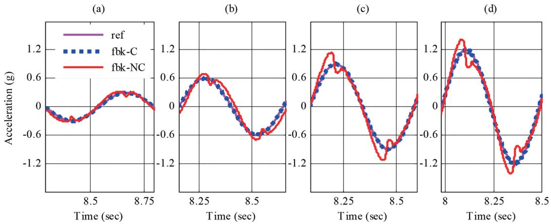
**Fig. 3** Shaking table reference (ref) and feedbacks, compensated (fbk-C) and uncompensated (fbk-NC), of harmonic tests at 2 Hz, performed whit peak amplitudes of (a) 0.30; (b) 0.60; (c) 0.90 and (d) 1.20g
