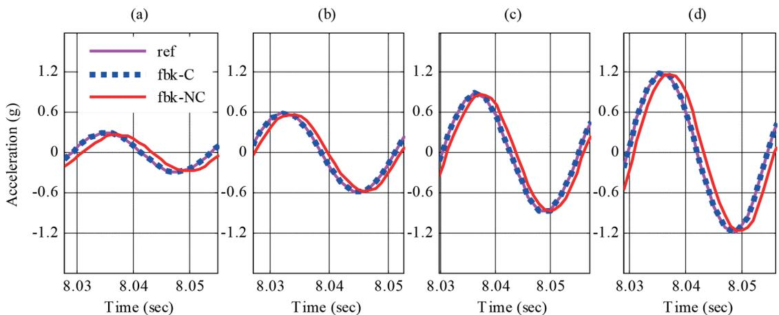
**Fig. 5** Shaking table reference (ref) and feedbacks, compensated (fbk-C) and uncompensated (fbk-NC), of harmonic tests at 40 Hz, performed whit peak amplitudes of (a) 0.30; (b) 0.60; (c) 0.90 and (d) 1.20g
