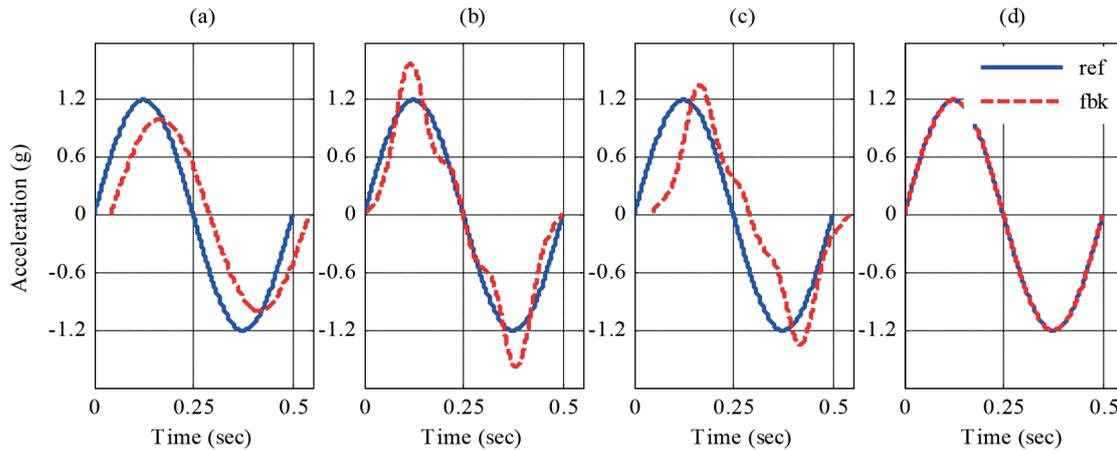
Fig. 2 Type of discrepancies in the shaking table feedbacks, (a) Amplitude and phase errors (b) Spurious harmonics (c) a and b combined (d) Ideal case
