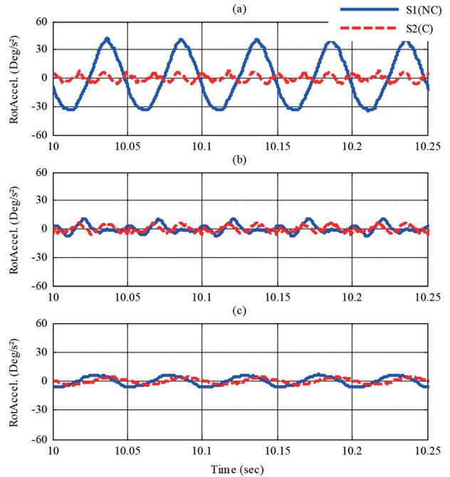
**Fig. 12** Rotational accelerations achieved on the CGS shaking table, (a): Roll, (b): Pitch and (c): Yaw, for sinusoidal tests S1 and S2
