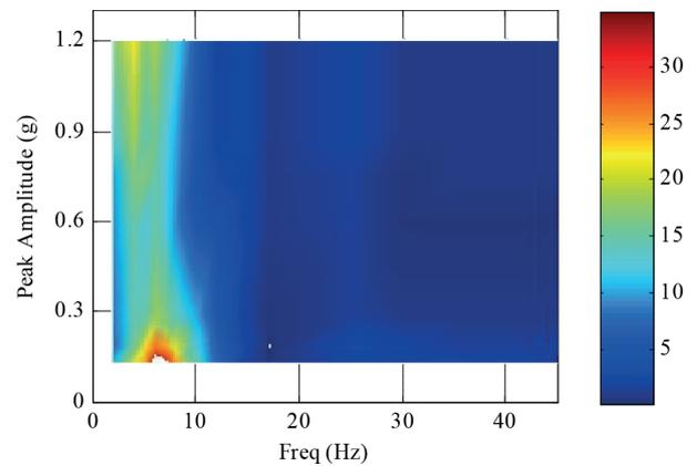
**Fig. 8** Total harmonic distortion of uncompensated set
