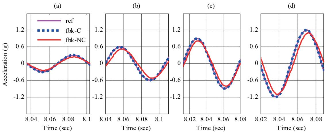
**Fig. 4** Shaking table reference (ref) and feedbacks, compensated (fbk-C) and uncompensated (fbk-NC), of harmonic tests at 15 Hz, performed whit peak amplitudes of (a) 0.30; (b) 0.60; (c) 0.90 and (d) 1.20g
