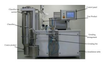
Fig. 1 Alpine Turboplex - Ultrafine Classifier 50 ATP, prepared in collaboration with [26]
